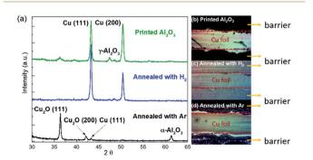
Fig. 2 (a) XRD of as printed, hydrogen-annealed, and argon-annealed Al<sub>2</sub>O<sub>3</sub>. (b-d) Corresponding optical micrographs of the barrier/graphene interface as printed (b), after 20 minute hydrogen-annealing (c), and 20 minute argon-annealed (d).
