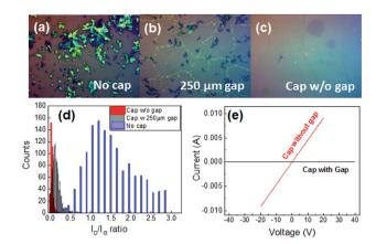
Fig. 4 OM images of graphene adjacent to the barrier after 6 hour graphene growth: (a) without cap, (b and c) with caps of different gap sizes (d) comparison of Raman  $I_{\rm D}/I_{\rm G}$  statistical distribution for graphene grown adjacent to the barriers using no cap, cap with 250  $\mu$ m spacing and directly covered cap (e) I-V characteristics of 1  $\times$  1 cm graphene devices grown under different gap sizes showing an increase in conductivity of  $10^6$  for confined-annealing.
