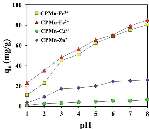
Fig. 6 The effects of pH on the adsorption of Fe<sup>3+</sup>, Fe<sup>2+</sup>, Ca<sup>2+</sup> and Zn<sup>2+</sup> by CP modified with KMnO<sub>4</sub>.
