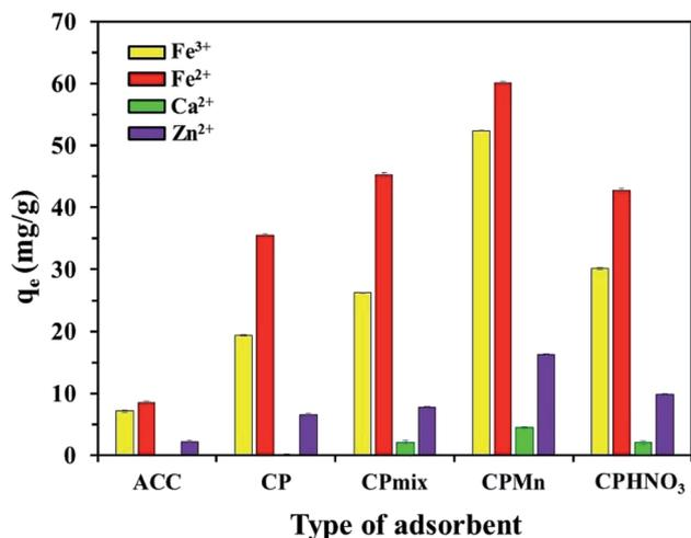
Fig. 1 A comparison of the Fe<sup>3+</sup>, Fe<sup>2+</sup>, Ca<sup>2+</sup> and Zn<sup>2+</sup> adsorption efficiencies using various adsorbents before and after modification with KMnO<sub>4</sub> and HNO<sub>3</sub>.
