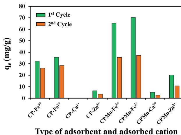
Fig. 8 Reusability of CP modified with KMnO<sub>4</sub> for the adsorption of Fe<sup>3+</sup>, Fe<sup>2+</sup>, Ca<sup>2+</sup> and Zn<sup>2+</sup>.
