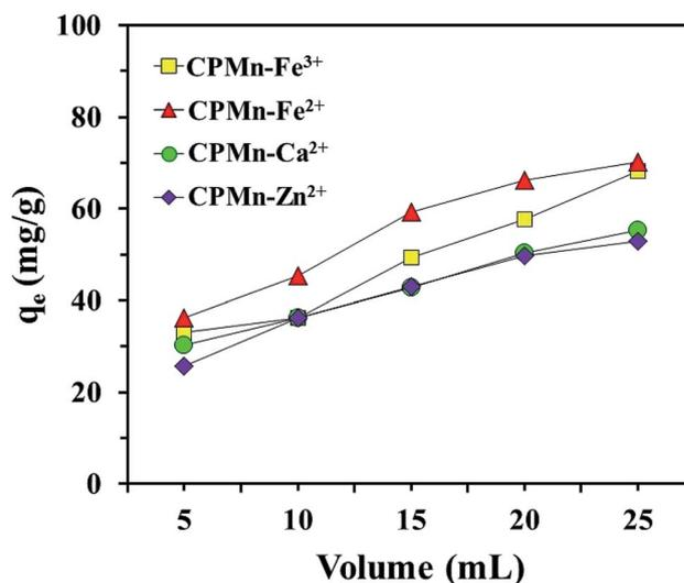
Fig. 7 The desorption of Fe<sup>3+</sup>, Fe<sup>2+</sup>, Ca<sup>2+</sup> and Zn<sup>2+</sup> from CP modified with KMnO<sub>4</sub> using different volumes of 1.0 mol L<sup>-1</sup> HNO<sub>3</sub>.
