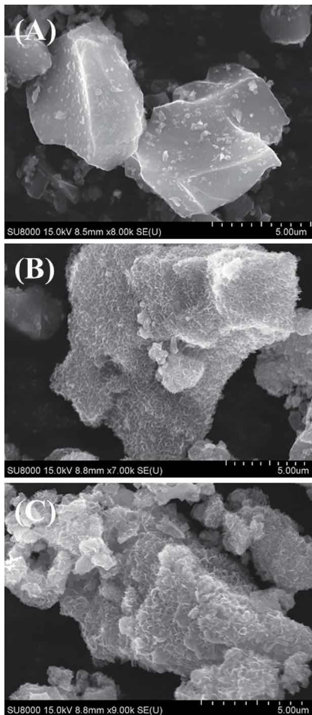
Fig. 5 SEM images of (A) CP, (B) CPMn and (C) CPMn after the Fe<sup>3+</sup> adsorption process.
