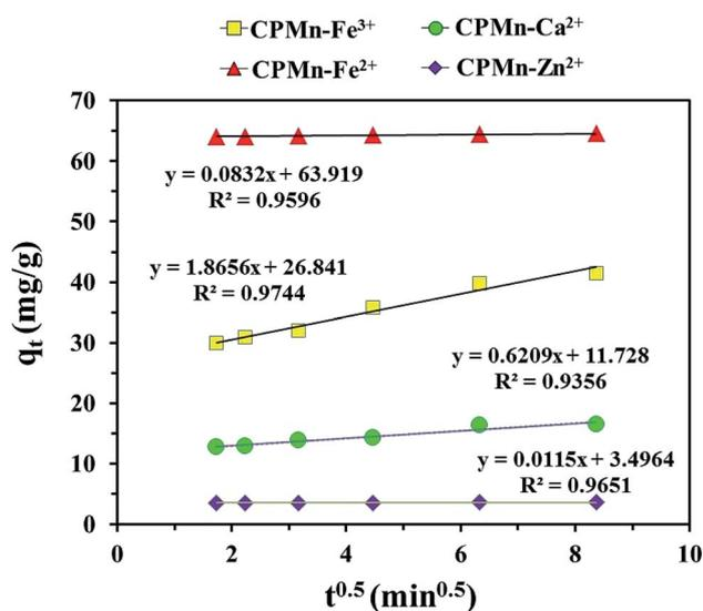
**Fig. 11** Intra-particle diffusion plots for  $\text{Fe}^{3+}$ ,  $\text{Fe}^{2+}$ ,  $\text{Ca}^{2+}$  and  $\text{Zn}^{2+}$  adsorption onto CPMn. The relative combined expanded uncertainty tSE is  $< \pm 0.02 \text{ mg g}^{-1}$  (0.95 level of confidence).
