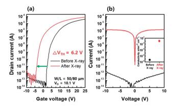
Fig. 2 (a) Transfer characteristics of an amorphous In-Ga-Zn-O (a-IGZO) thin film transistor (TFT) before (black line) and after (red line) Xray irradiation. (b) Increase in current level and conductivity (inset) of the active layer before (black line) and after (red line) X-ray irradiation.
