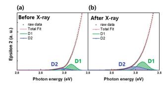
Fig. 4 Spectroscopic ellipsometry (SE) spectra of the dielectric function ( $\varepsilon_2$ ) deconvoluted for two sub-gap states (denoted as D1 and D2) of the amorphous In–Ga–Zn–O (a-IGZO) film (a) before and (b) after X-ray irradiation. The two sub-gap states located near the conduction band minima were deconvoluted with a Gaussian fit. Both relative areas of the sub-gap states increased after X-ray irradiation.
