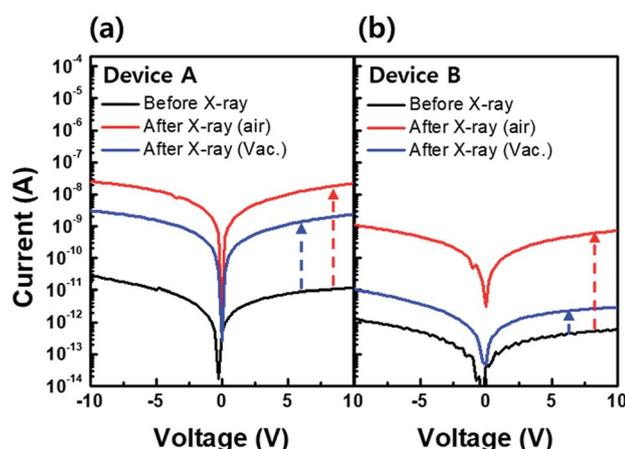
Fig. 5 Current level variation of (a) device A (with hydrogen rich buffer layer) and (b) device B (without buffer layer) before (black line) and after X-ray irradiation in air (red line) and ambient vacuum (blue line). Device A shows more increase in current level after X-ray irradiation in air and ambient vacuum compared to that in device B. Both devices show less increase in current level in ambient vacuum irradiation compared to air ambient irradiation.
