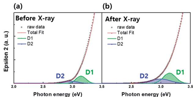
Fig. 4 Spectroscopic ellipsometry (SE) spectra of the dielectric function ( $\epsilon_2$ ) deconvoluted for two sub-gap states (denoted as D1 and D2) of the amorphous In–Ga–Zn–O (a-IGZO) film (a) before and (b) after X-ray irradiation. The two sub-gap states located near the conduction band minima were deconvoluted with a Gaussian fit. Both relative areas of the sub-gap states increased after X-ray irradiation.
