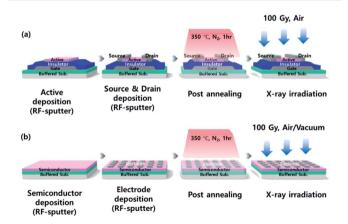
Fig. 1 Schematic flows of the fabrication of (a) a bottom-gated amorphous In-Ga-Zn-O (a-IGZO) thin film transistor (TFT) and (b) film type a-IGZO sample. In the device, Mo is used as a gate, SiO<sub>2</sub> is used as a gate insulator, a-IGZO is used as an active layer (semiconductor), and In-Sn-O (ITO) is used as source and drain top electrodes.
