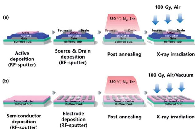
Fig. 1 Schematic flows of the fabrication of (a) a bottom-gated amorphous In-Ga-Zn-O (a-IGZO) thin film transistor (TFT) and (b) film type a-IGZO sample. In the device, Mo is used as a gate,  $\text{SiO}_2$  is used as a gate insulator, a-IGZO is used as an active layer (semiconductor), and In-Sn-O (ITO) is used as source and drain top electrodes.
