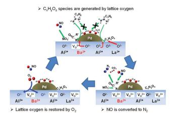
Fig. 8 Presumed reaction scheme for NO reduction on Pd/  $La_{0.9}Ba_{0.1}AlO_{3-\delta}.$
