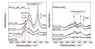
Fig. 6 DRIFT spectra of Pd/La $_{0.9}$ Ba $_{0.1}$ AlO $_{3-\delta}$  and Pd/Ba/LaAlO $_{3}$  during transient test (switching from C<sub>3</sub>H<sub>6</sub> to O<sub>2</sub> flow).
