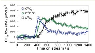
Fig. 4 Transient response curves for typical products on Pd/La $_{0.9}$ -Ba $_{0.1}$ AlO $_{3-\delta}$  following Ar  $\to$  C $_3$ H $_6$  +  $^{18}$ O $_2$  switch at 523 K.
