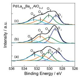
Fig. 5 XP spectra of O1s for Pd/La $_{0.9}$ Ba $_{0.1}$ AlO $_{3-\delta}$  (a) after exposure in C<sub>3</sub>H<sub>6</sub> flow, (b) after exposure in O<sub>2</sub> and (c) after exposure of C<sub>3</sub>H<sub>6</sub> flow again.
