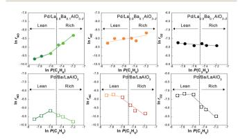
Fig. 3 Dependence of the reaction rate on the partial pressure of  $C_3H_6$ on Pd/La<sub>0.9</sub>Ba<sub>0.1</sub>AlO<sub>3- $\delta$ </sub> and Pd/Ba/LaAlO<sub>3</sub> at 523 K during NO-C<sub>3</sub>H<sub>6</sub>-O2-H2O reaction.
