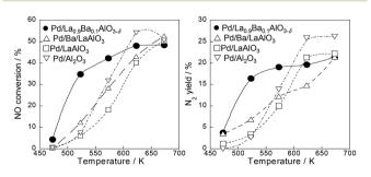
Fig. 1 Comparison of NO conversions and N<sub>2</sub> yields over Pd/La<sub>0.9</sub>- $Ba_{0.1}AlO_{3-\delta}$ , Pd/Ba/LaAlO<sub>3</sub>, Pd/LaAlO<sub>3</sub> and Pd/Al<sub>2</sub>O<sub>3</sub>. Reaction conditions: total flow rate =  $200 \text{ mL min}^{-1}$ , NO 1000 ppm,  $C_3H_6$  500 ppm, O<sub>2</sub> 2000 ppm, H<sub>2</sub>O 7 vol%.
