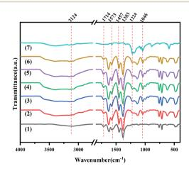
Fig. 2 The FT-IR spectra of MIL-100(Fe) (1), X-[PrSO<sub>3</sub>HMIm]HSO<sub>4</sub>@-MIL-100(Fe) (2-6) (X = 0.7, 0.9, 1.1, 1.3, 1.5) and [PrSO<sub>3</sub>HMIm]HSO<sub>4</sub> (7).
