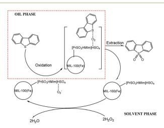
Scheme 1 Proposed mechanism of coupled oxidation extraction desulfurization.
