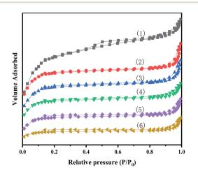
Fig. 3  $N_2$  adsorption–desorption isotherms for MIL-100(Fe) (1) and X- $[PrSO_3HMIm]HSO_4@MIL-100(Fe)$  (2-6) (X = 0.7, 0.9, 1.1, 1.3, 1.5).
