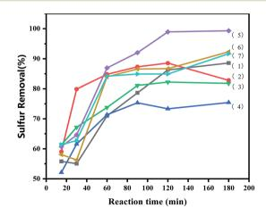
Fig. 4 Effects of reaction time and loading amount of IL on oxidative desulfurization. (1) [PrSO<sub>3</sub>HMIm]HSO<sub>4</sub>, (2) MIL-100(Fe), (3-7) X-ILs@-MIL-100(Fe) (X = 0.7, 0.9, 1.1, 1.3, 1.5), the following conditions were used: catalyst, 0.05 g; model oil, 10 mL; acetonitrile, 10 mL; H<sub>2</sub>O<sub>2</sub>, 28 μL; t, 180 min; T, 60 °C.
