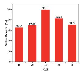
Fig. 6 Effects of  $H_2O_2/DBT$  ratio on oxidative desulfurization. The experiments were conducted under the following conditions: catalyst, 0.05 g; model oil, 10 mL; acetonitrile, 10 mL; t, 180 min; T, 60 °C.
