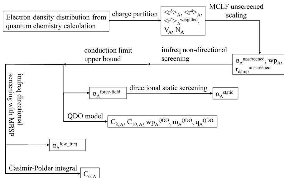
**Fig. 9** Flow diagram for MCLF method.
