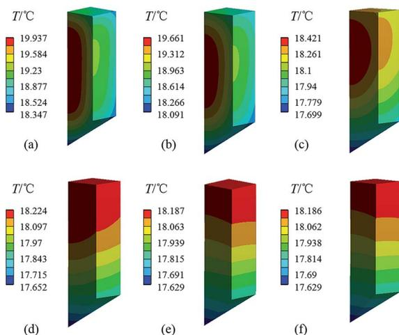
Fig. 4 Temperature distribution in the 0.5 m KDP crystal at different times after the growth was completed, in the case of extracting the solution: (a) 3 h; (b) 6 h; (c) 24 h; (d) 36 h; (e) 72 h; (f) steady-state.
