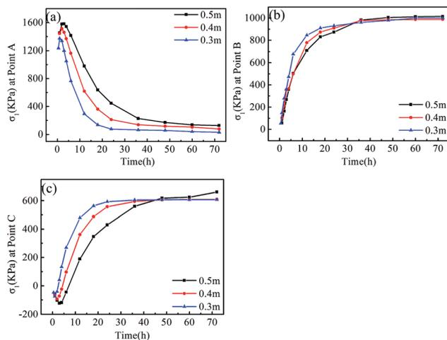
Fig. 7 The maximum  $\sigma_1$  evolution at the outside surface (point A), the interior (point B) and the top end of the cap region (point C) of the three sizes of crystals in the case of extracting the solution.
