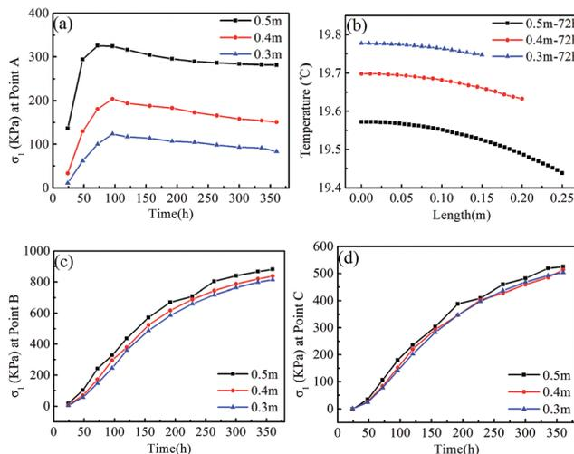
Fig. 12 The evolution of maximum  $\sigma_1$  at different positions in the three sizes of crystals and the temperature profile at the time at which peak  $\sigma_1$  is a maximum, in the case of retaining the solution: (a) point A, (b) temperature profile along the path of EF, labelled in Fig. 2b, (c) point B and (d) point C.
