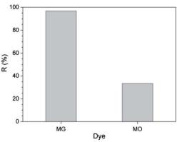
Fig. 4 Separation of malachite green (MG) and methyl orange (MO) by flotation with HeSat as the collector. Conditions:  $c_{\text{HeSat}} = 0.5 \text{ g L}^{-1}$ ,  $c_{\text{MG}} = c_{\text{MO}} = 10 \text{ mg L}^{-1}$ , 13.4 ml min<sup>-1</sup> N<sub>2</sub>, and t = 4 h. Left: colours of the dye solution before (A) and after (B) the flotation experiment, right: dye removal efficiencies. Reproduced from ref. 51 with permission from Elsevier, Copyright 2017.
