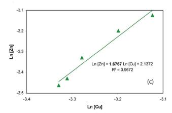
Fig. 10 Ion flotation selectivity coefficient determination: Cd and Zn (a), Cd and Cu (b), Zn and Cu (c). Adapted from ref. 96 with permission. Copyright 2013 American Chemical Society.
