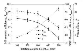
Fig. 5 Effects of flotation column height on  $R_{\rm MB}$ ,  $R_{\rm SNPs}$  and  $\varphi$ . Reproduced from ref. 52 with permission from Springer, Copyright 2017. Reprinted by permission from Springer, N. Hu, W. Liu, L. Ding, Z. Wu, H. Yin, D. Huang, H. Li, L. Jin and H. Zheng, Removal of methylene blue from its aqueous solution by froth flotation: hydrophobic silica nanoparticle as a collector, *J. Nanopart. Res.*, Copyright (2017).
