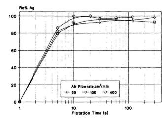
Fig. 7 Effects of flotation time and air flowrate on  $R_{Ag}$ . Reproduced from ref. 80 with permission from Elsevier, Copyright 1995. Reprinted from A. I. Zouboulis, Silver recovery from aqueous streams using ion flotation, *Miner. Eng.*, **8**, 1477–1488, Copyright (1995), with permission from Elsevier.
