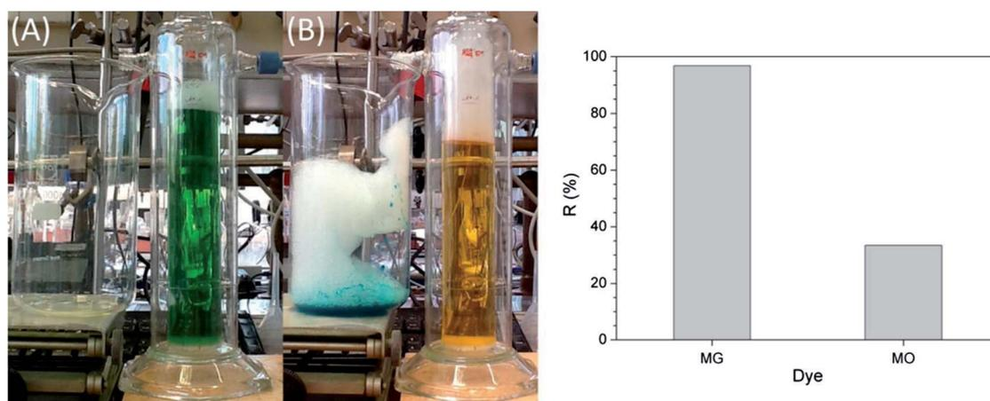
Fig. 4 Separation of malachite green (MG) and methyl orange (MO) by flotation with HeSat as the collector. Conditions:  $c_{\text{HeSat}} = 0.5 \text{ g L}^{-1}$ ,  $c_{\text{MG}} = c_{\text{MO}} = 10 \text{ mg L}^{-1}$ ,  $13.4 \text{ ml min}^{-1} \text{ N}_2$ , and  $t = 4 \text{ h}$ . Left: colours of the dye solution before (A) and after (B) the flotation experiment, right: dye removal efficiencies. Reproduced from ref. 51 with permission from Elsevier, Copyright 2017.
