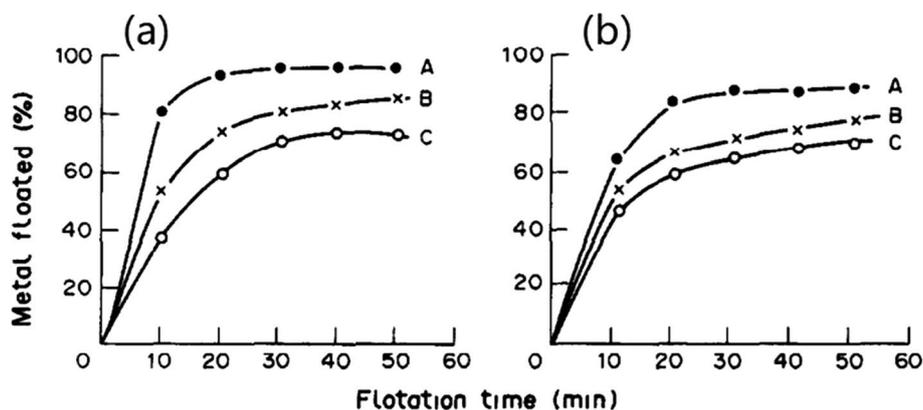
Fig. 8 Effects of flotation time and surfactants on  $R_{Rh}$  (a),  $R_{Pd}$  (b) recovery: A SDBS, B SDS, C sodium lauryl sulfate (SLS). Reproduced from ref. 13 with permission from Elsevier, Copyright 1991. Reprinted from X. He, Ion flotation of rhodium(III) and palladium(II) with anionic surfactants, *Talanta*, **38**, 319–323, Copyright (1991), with permission from Elsevier.
