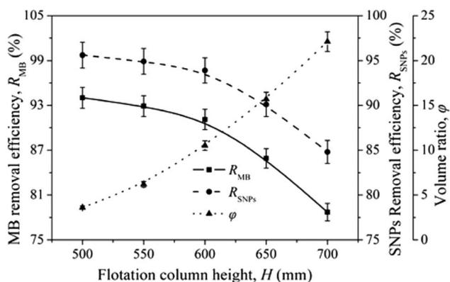
Fig. 5 Effects of flotation column height on  $R_{\text{MB}}$ ,  $R_{\text{SNPs}}$  and  $\phi$ . Reproduced from ref. 52 with permission from Springer, Copyright 2017. Reprinted by permission from Springer, N. Hu, W. Liu, L. Ding, Z. Wu, H. Yin, D. Huang, H. Li, L. Jin and H. Zheng, Removal of methylene blue from its aqueous solution by froth flotation: hydrophobic silica nanoparticle as a collector, *J. Nanopart. Res.*, Copyright (2017).
