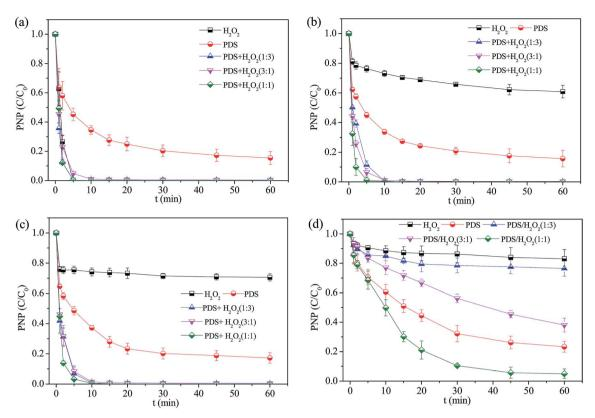
Fig. 4 PNP degradation in different oxidation systems with different initial pH (a) pH = 3, (b) pH = 5, (c) pH = 7, (d) pH = 10. Reaction condition:  $[nZVI]_0 = 0.2 \text{ g L}^{-1}$ ,  $[PNP]_0 = 20 \text{ mg L}^{-1}$ ,  $[H_2O_2]_0 = 2 \text{ mmol L}^{-1}$ ,  $[PDS]_0 = 2 \text{ mmol L}^{-1}$ ,  $[H_2O_2/PDS]_0 = 2 \text{ mmol L}^{-1}$ .
