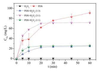
Fig. 5 Concentration of leached iron in nZVI/H $_2$ O $_2$ , nZVI/PDS and nZVI/H $_2$ O $_2$ /PDS systems. Reaction condition: [nZVI] $_0=0.2~\rm g~L^{-1}$ , [PNP] $_0=20~\rm mg~L^{-1}$ , [H $_2$ O $_2$ ] $_0=$  [PDS] $_0=2~\rm mM$ , [H $_2$ O $_2$ /PDS (1 : 1)] $_0=2~\rm mmol~L^{-1}$ , initial pH = 7.
