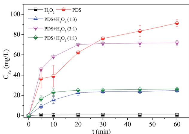
Fig. 5 Concentration of leached iron in nZVI/H<sub>2</sub>O<sub>2</sub>, nZVI/PDS and nZVI/H<sub>2</sub>O<sub>2</sub>/PDS systems. Reaction condition: [nZVI]<sub>0</sub> = 0.2 g L<sup>-1</sup>, [PNP]<sub>0</sub> = 20 mg L<sup>-1</sup>, [H<sub>2</sub>O<sub>2</sub>]<sub>0</sub> = [PDS]<sub>0</sub> = 2 mM, [H<sub>2</sub>O<sub>2</sub>/PDS (1 : 1)]<sub>0</sub> = 2 mmol L<sup>-1</sup>, initial pH = 7.
