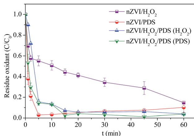
Fig. 2 Oxidants consumption in nZVI/ $\text{H}_2\text{O}_2$ , nZVI/PDS and nZVI/ $\text{H}_2\text{O}_2$ /PDS systems. Reaction condition:  $[\text{nZVI}]_0 = 0.2 \text{ g L}^{-1}$ ,  $[\text{PNP}]_0 = 20 \text{ mg L}^{-1}$ ,  $[\text{PDS}]_0 = [\text{H}_2\text{O}_2]_0 = 2 \text{ mM}$ ,  $[\text{H}_2\text{O}_2/\text{PDS} (1 : 1)]_0 = 2 \text{ mmol L}^{-1}$ , initial pH = 7.
