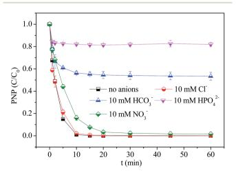
Fig. 7 The effect of water matrices on PNP degradation in the nZVI/  $H_2O_2/PDS$  system. Reaction condition:  $[nZVI]_0 = 0.2 \text{ g L}^{-1}$ ,  $[PNP]_0 =$ 20 mg L<sup>-1</sup>,  $[H_2O_2/PDS (1 : 1)]_0 = 2$  mM.
