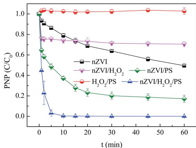
Fig. 1 Degradation of PNP in different reaction systems. Reaction condition:  $[\text{PNP}]_0 = 20 \text{ mg L}^{-1}$ ,  $[\text{H}_2\text{O}_2]_0 = 2 \text{ mmol L}^{-1}$ ,  $[\text{PDS}]_0 = 2 \text{ mmol L}^{-1}$ ,  $[\text{H}_2\text{O}_2/\text{PDS}]_0 = 2 \text{ mmol L}^{-1}$ ,  $[\text{nZVI}]_0 = 0.2 \text{ g L}^{-1}$ , initial pH = 7. Note: in the nZVI/ $\text{H}_2\text{O}_2$ /PDS system, the molar ratio of  $\text{H}_2\text{O}_2$ /PDS was 1.
