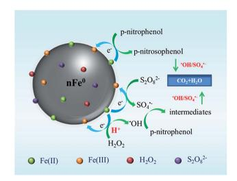
Fig. 9 Proposed mechanisms for simultaneous activation of  $H_2O_2/PDS$  with nZVI as the activator.
