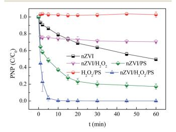
Fig. 1 Degradation of PNP in different reaction systems. Reaction condition:  $[\text{PNP}]_0=20\,\text{mg}\,\text{L}^{-1},\ [\text{H}_2\text{O}_2]_0=2\,\text{mmol}\,\text{L}^{-1},\ [\text{PDS}]_0=2\,\text{mmol}\,\text{L}^{-1},\ [\text{H}_2\text{O}_2/\text{PDS}]_0=2\,\text{mmol}\,\text{L}^{-1},\ [\text{InZVI}]_0=0.2\,\text{g}\,\text{L}^{-1},\ \text{initial}\,\text{pH}=7.$  Note: in the nZVI/H<sub>2</sub>O<sub>2</sub>/PDS system, the molar ratio of H<sub>2</sub>O<sub>2</sub>/PDS was 1.
