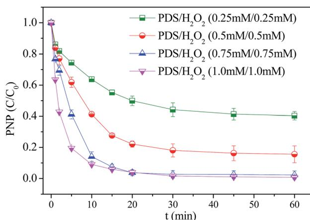
Fig. 6 PNP degradation in the nZVI/H<sub>2</sub>O<sub>2</sub>/PDS system with different oxidant dosage. Reaction condition: [nZVI]<sub>0</sub> = 0.2 g L<sup>-1</sup>, [PNP]<sub>0</sub> = 20 mg L<sup>-1</sup>, [H<sub>2</sub>O<sub>2</sub>]<sub>0</sub>/[PDS]<sub>0</sub> = 1 : 1, initial pH = 7.
