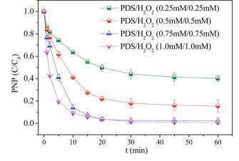
Fig. 6 PNP degradation in the nZVI/H<sub>2</sub>O<sub>2</sub>/PDS system with different oxidant dosage. Reaction condition:  $[nZVI]_0 = 0.2 \text{ g L}^{-1}$ ,  $[PNP]_0 = 20 \text{ mg L}^{-1}$ ,  $[H_2O_2]_0/[PDS]_0 = 1:1$ , initial pH = 7.
