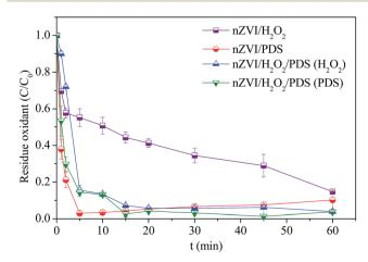
Fig. 2 Oxidants consumption in nZVI/H<sub>2</sub>O<sub>2</sub>, nZVI/PDS and nZVI/H<sub>2</sub>O<sub>2</sub>/PDS systems. Reaction condition: [nZVI]<sub>0</sub> = 0.2 g L<sup>-1</sup>, [PNP]<sub>0</sub> = 20 mg L<sup>-1</sup>, [PDS]<sub>0</sub> = [H<sub>2</sub>O<sub>2</sub>]<sub>0</sub> = 2 mM, [H<sub>2</sub>O<sub>2</sub>/PDS (1 : 1)]<sub>0</sub> = 2 mmol L<sup>-1</sup>, initial pH = 7.
