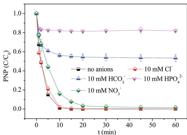
Fig. 7 The effect of water matrices on PNP degradation in the nZVI/ $\text{H}_2\text{O}_2$ /PDS system. Reaction condition:  $[\text{nZVI}]_0 = 0.2 \text{ g L}^{-1}$ ,  $[\text{PNP}]_0 = 20 \text{ mg L}^{-1}$ ,  $[\text{H}_2\text{O}_2/\text{PDS} (1 : 1)]_0 = 2 \text{ mM}$ .
