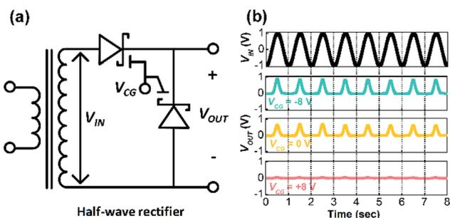
Fig. 4 (a) Circuit diagram and (b) sequential measurement results of a half-wave rectifier circuit with two flexible CNT Schottky diodes for  $V_{CG}$  values of  $-8$  V,  $0$  V, and  $+8$  V.
