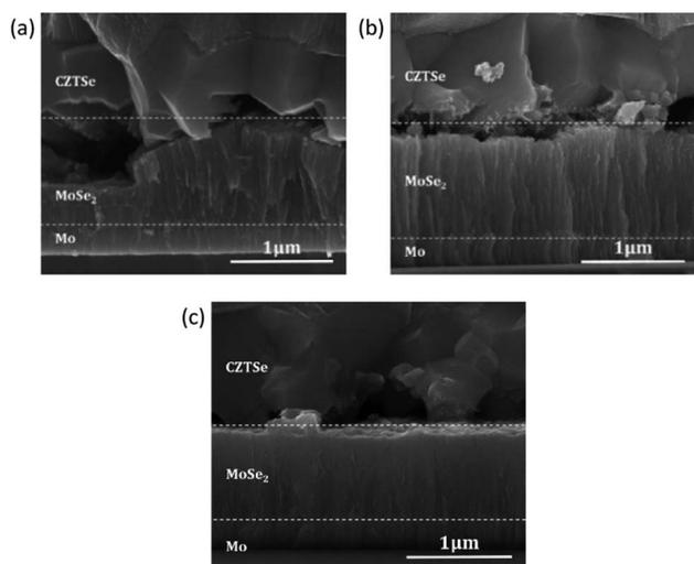
Fig. 3 SEM cross-section of CZTSe solar cells prepared on the Mo substrates (a) without plasma, (b) with Ar plasma and (c) with Ar–N<sub>2</sub> plasma treatments.
