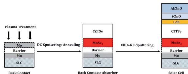
Fig. 2 Standard fabrication process of CZTSe solar cells in this study.
