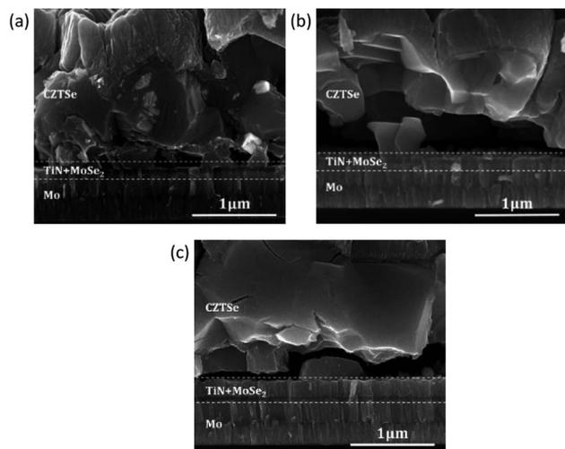
Fig. 6 SEM cross-section of CZTSe solar cells with TiN back-contact barriers: (a) Mo/TiN back contact without plasma treatment, (b) Mo/TiN back contact with Ar plasma treatment and (c) Mo/TiN/Mo back contact with Ar plasma treatment.
