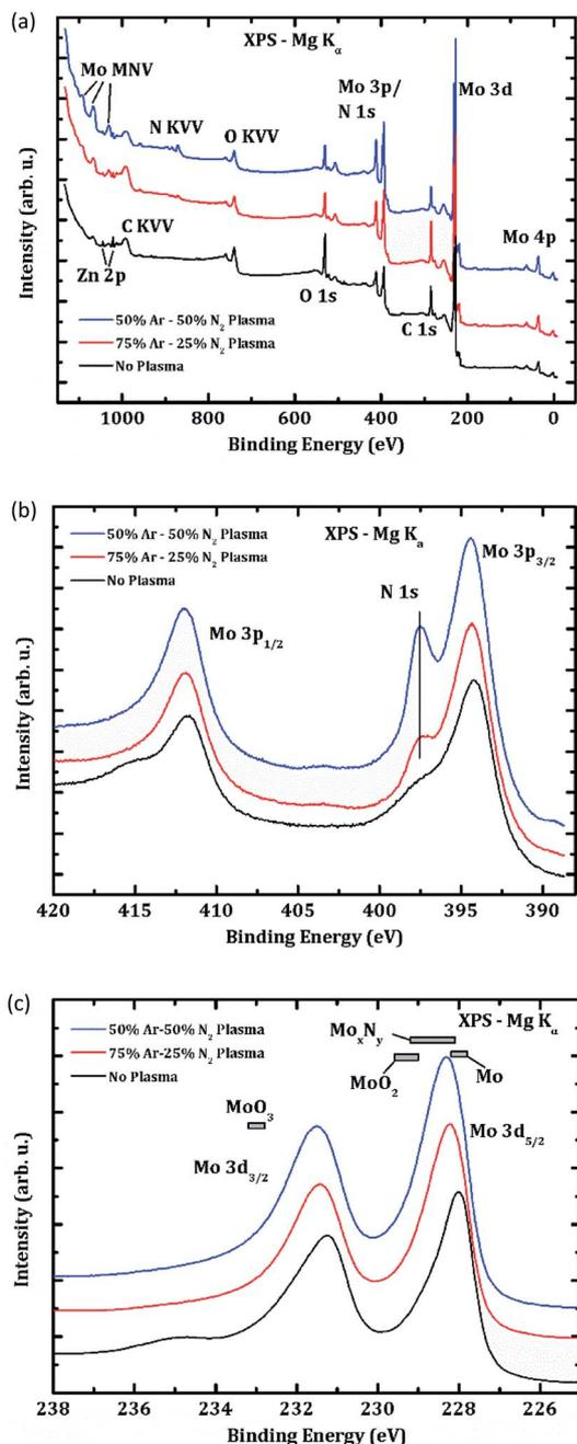
Fig. 5 (a) XPS survey spectra, (b) Mo 3p and N 1s spectrum, and (c) Mo 3d spectrum of Mo substrates. Black spectra were recorded for a sample without Ar-N<sub>2</sub> plasma treatment, red and blue spectra were collected after an Ar-N<sub>2</sub> plasma treatment with an Ar/N ratio of 75/25 and 50/50, respectively.
