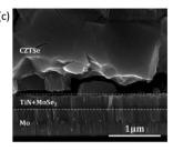
Fig. 6 SEM cross-section of CZTSe solar cells with TiN back-contact barriers: (a) Mo/TiN back contact without plasma treatment, (b) Mo/TiN back contact with Ar plasma treatment and (c) Mo/TiN/Mo back contact with Ar plasma treatment.
