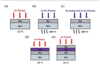
Fig. 1 Back-contact modifications with plasma treatments in this study: (a) Mo with Ar plasma, (b) Mo with Ar $-N_2$  plasma, (c) Mo with  $N_2$ enhanced Ar-N<sub>2</sub> plasma, (d) Mo/TiN with Ar plasma and (e) Mo/TiN/ Mo with Ar plasma.
