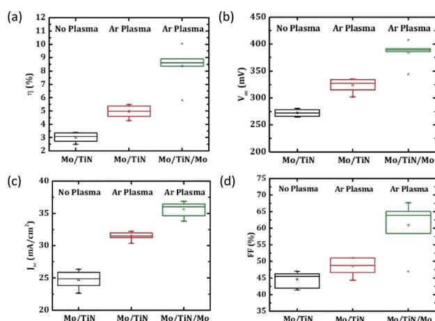
Fig. 7 Box plots of solar cell parameters (a) energy conversion efficiency  $\eta$ , (b) open circuit voltage  $V_{oc}$ , (c) short circuit current density  $J_{sc}$  and (d) fill factor FF for the samples with TiN back contact barriers. For every type of back contacts, 6 cells are included.
