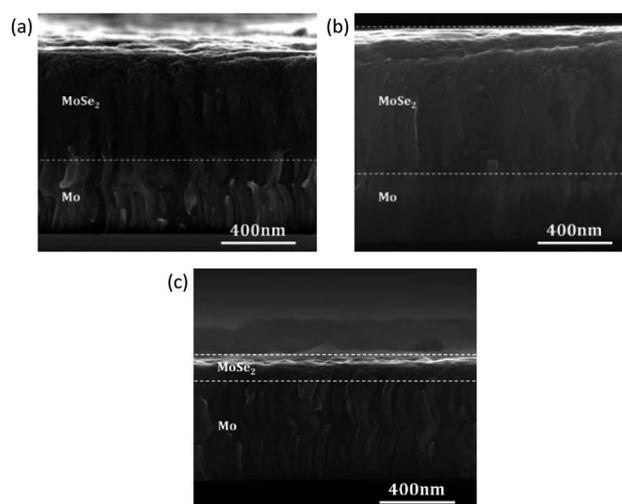
Fig. 4 SEM cross-section of selenized bare Mo substrates (a) without plasma, (b) with Ar plasma and (c) with Ar–N<sub>2</sub> plasma treatments.
