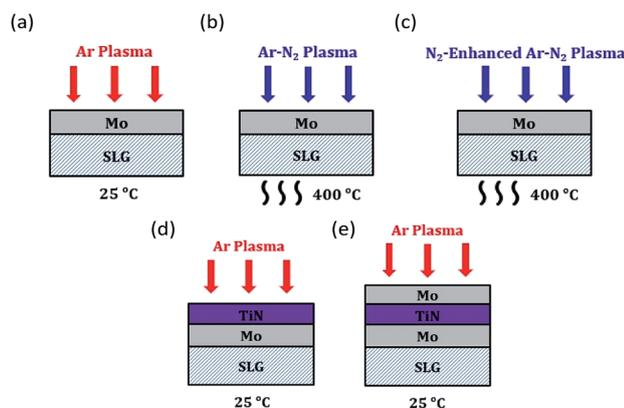
Fig. 1 Back-contact modifications with plasma treatments in this study: (a) Mo with Ar plasma, (b) Mo with Ar–N<sub>2</sub> plasma, (c) Mo with N<sub>2</sub>-enhanced Ar–N<sub>2</sub> plasma, (d) Mo/TiN with Ar plasma and (e) Mo/TiN/Mo with Ar plasma.
