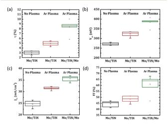
Fig. 7 Box plots of solar cell parameters (a) energy conversion efficiency  $\eta$ , (b) open circuit voltage  $V_{\rm oc}$ , (c) short circuit current density  $J_{\rm sc}$  and (d) fill factor FF for the samples with TiN back contact barriers. For every type of back contacts, 6 cells are included.
