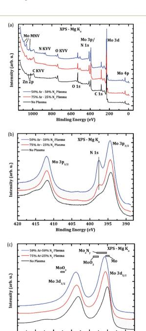
Fig. 5 (a) XPS survey spectra, (b) Mo 3p and N 1s spectrum, and (c) Mo 3d spectrum of Mo substrates. Black spectra were recorded for a sample without  $Ar-N_2$  plasma treatment, red and blue spectra were collected after an  $Ar-N_2$  plasma treatment with an Ar/N ratio of 75/25 and 50/50, respectively.
