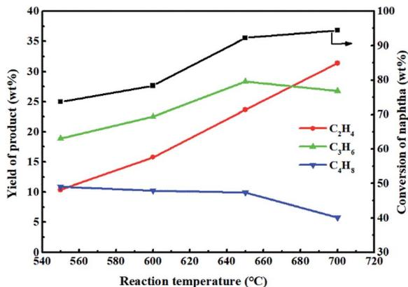
Fig. 12 Effect of reaction temperature on the reactivity of 0.3-ZnZSM-5 in the methanol promoted naphtha catalytic pyrolysis system. Reaction conditions: methanol/naphtha = 15 wt%, WHSV = 3.83 h<sup>-1</sup>, N<sub>2</sub> = 60 mL min<sup>-1</sup>, time on stream = 3 h.
