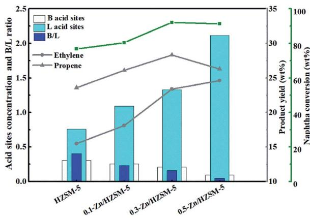
Fig. 10 Effect of acidity on the catalytic reactivity of Zn/HZSM-5 in the methanol promoted naphtha catalytic pyrolysis system. Reaction conditions: reaction temperature = 650 °C, WHSV = 3.83 h<sup>-1</sup>, N<sub>2</sub> = 60 mL min<sup>-1</sup>, methanol/naphtha = 15 wt%, time on stream = 3 h.
