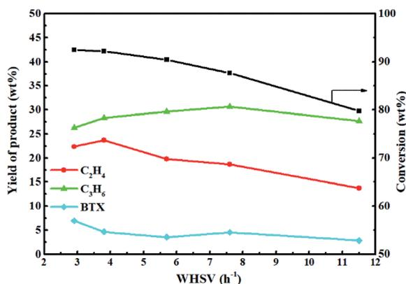
Fig. 13 Effect of WHSV on the reactivity of 0.3-ZnZSM-5 in the methanol promoted naphtha catalytic pyrolysis system. Reaction conditions: reaction temperature = 650 °C, methanol/naphtha = 15 wt%, N<sub>2</sub> = 60 mL min<sup>-1</sup>, time on stream = 3 h.
