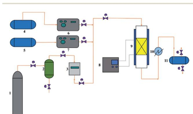
Fig. 1 Experimental setup for the catalytic performance evaluation. 1- N<sub>2</sub> cylinder, 2-desiccator, 3-mass flow controller, 4-naphtha container, 5-methanol container, 6-constant flux pump, 7-constant flux pump, 8-temperature controller, 9-fixed-bed reactor, 10-condenser, 11-liquid product container.
