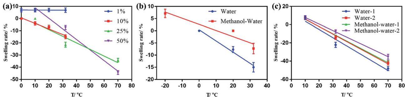
Fig. 3 (a) The relationship of swelling ratio and temperature of dual-responsive ONHs with 1, 10, 25 or 50% NiPAm addition; (b) the relationship of swelling ratio and temperature of dual-responsive ONHs with 10% of NiPAm addition in different environments; (c) the relationship of swelling ratio and temperature of dual-responsive ONHs with 50% NiPAm addition at different polymerization times.
