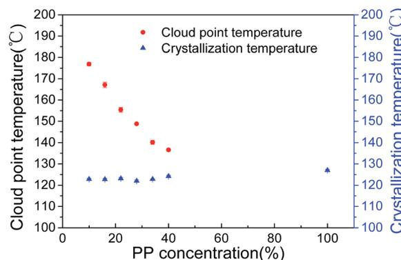
Fig. 1 Phase diagram for the PP/binary diluents system with various PP contents: diluents content (SO/CO): 84/16.
