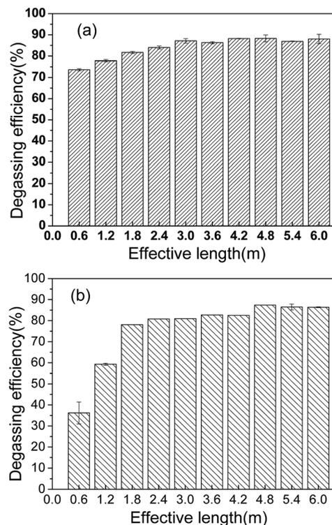
Fig. 8 Effect of effective length on degassing efficiency. (Operating conditions: initial CO<sub>2</sub> concentration of 16.5 mg L<sup>-1</sup>; vacuum degree of 0.095 MPa; flow rate of (a) 20 mL min<sup>-1</sup> and (b) 63 mL min<sup>-1</sup>).
