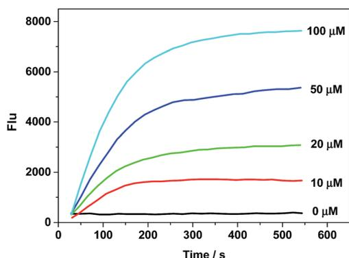
Fig. 2 Fluorescence intensity changes ( $F_{610\text{ nm}}$ ) with  $\lambda_{\text{ex}} = 450\text{ nm}$  at  $37\text{ }^\circ\text{C}$  over an incubation time of 10 min at varied concentrations of **AZO-Cy**: 0 (control), 10, 20, 50 and 100  $\mu\text{M}$ . The measurements were performed in PBS buffer with 1.0  $\text{U mL}^{-1}$  CPR and 100  $\mu\text{M}$  of NADH.
