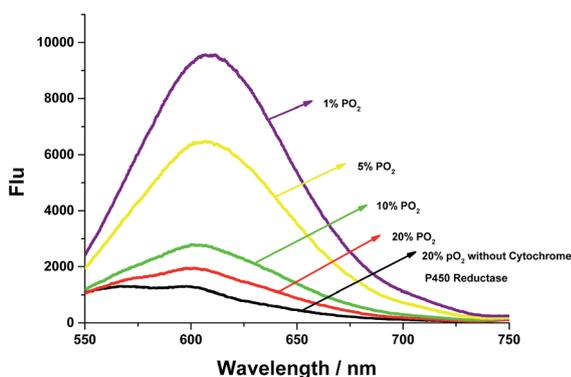
Fig. 3 Fluorescence changes of **AZO-Cy** without (purple curve) or with (other curves) various oxygen levels. The spectra were measured in phosphate buffer (pH 7.4 with 1% DMSO, containing 0.1 mM NADH) at  $37\text{ }^\circ\text{C}$ .
