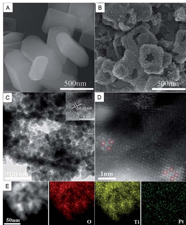
Fig. 2 SEM images of (A) NH<sub>4</sub>TiOF<sub>3</sub> mesocrystals and (B) 1% Pt/TiO<sub>2</sub>-TC catalysts. (C) A TEM image of 1% Pt/TiO<sub>2</sub>-TC; the inset shows the crystal lattice of anatase TiO<sub>2</sub>. (D) High-resolution HAADF-STEM images of 1% Pt/TiO<sub>2</sub>-TC. (E) EDS elemental mapping of a single 1% Pt/TiO<sub>2</sub>-TC crystal.
