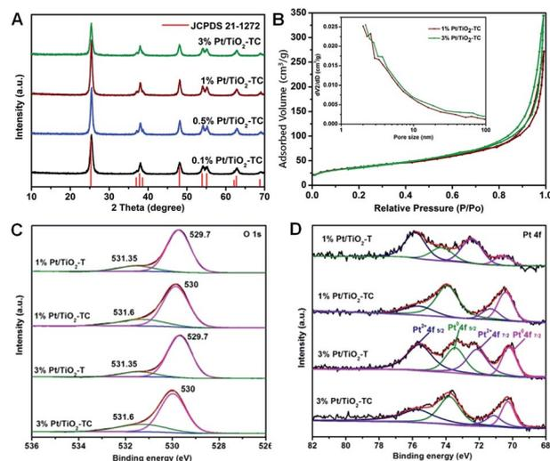
Fig. 3 (A) XRD patterns of Pt/TiO<sub>2</sub>-TC catalysts with different Pt loading content. (B) N<sub>2</sub> adsorption-desorption isotherms and pore size distributions (inset) of Pt/TiO<sub>2</sub>-TC catalysts. (C) O 1s XPS spectra and (D) Pt 4f XPS spectra for Pt/TiO<sub>2</sub> catalysts.
