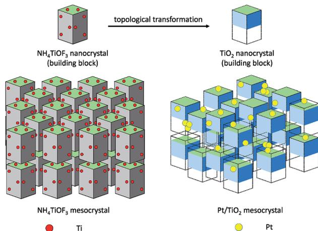
Fig. 1 Schematic diagram of the synthesis of Pt/TiO<sub>2</sub>-TC.
