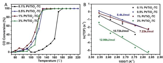
Fig. 4 (A) CO conversion and (B) corresponding Arrhenius plots of the reaction rate  $\ln(\text{TOF})$  versus  $1/T$  for the CO oxidation reaction using Pt/TiO<sub>2</sub>-TC catalysts with different Pt loading content.
