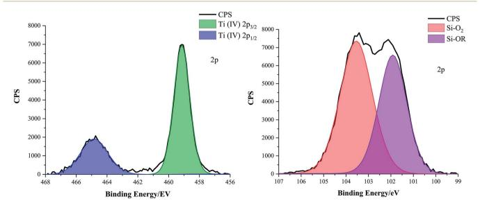
Fig. 3 Deconvoluted X-ray photoelectron spectroscopy (XPS) Ti 2p and Si 2p scans of coating D comprising SiO<sub>2</sub>  $5-15 \mu m$  particles (0.6 g) and TiO<sub>2</sub> 21 nm particles (0.6 g) in a 1 : 9 polymer mixture of Sylgard® 184 and FAS.
