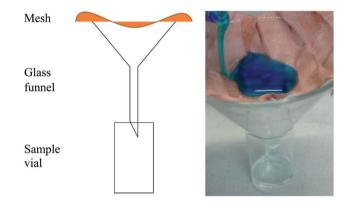
Fig. 2 Schematic and image of solvent—water separation efficiency apparatus. Mixtures of known compositions were poured onto various coated sample meshes. The mass of solvent collected after 30 s of separation provided relevant information for the calculation of a comparable separation efficiency percentage.
