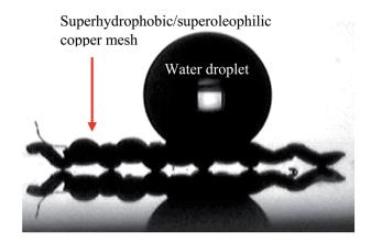
Fig. 8 Water droplet on a copper 60 mesh substrate with a coating D surface ( $SiO_2 5-15 \mu m$  particles (0.6 g) with  $TiO_2 21 nm$  particles (0.6 g) in a 1:9 polymer mixture of Sylgard® 184 and FAS). Image was recorded post separation functional testing.
