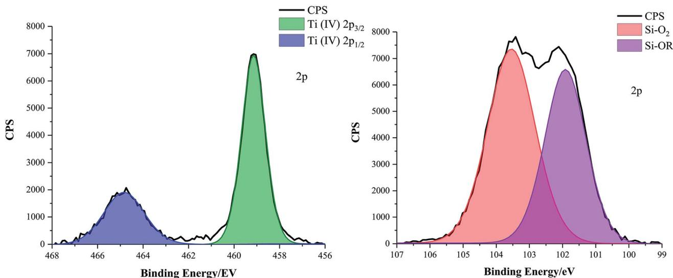
Fig. 3 Deconvoluted X-ray photoelectron spectroscopy (XPS) Ti 2p and Si 2p scans of coating D comprising SiO<sub>2</sub> 5–15 μm particles (0.6 g) and TiO<sub>2</sub> 21 nm particles (0.6 g) in a 1 : 9 polymer mixture of Sylgard® 184 and FAS.
