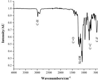
Fig. 4 Fourier transform infrared (FT-IR) spectrum of coating D; SiO<sub>2</sub> 5-15  $\mu$ m particles (0.6 g) and TiO<sub>2</sub> 21 nm particles (0.6 g) in a 1:9 polymer mixture of Sylgard® 184 and FAS.
