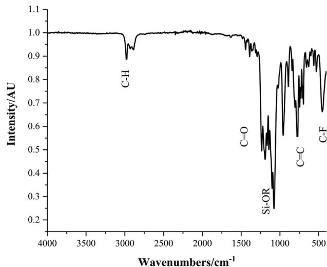
Fig. 4 Fourier transform infrared (FT-IR) spectrum of coating D; SiO<sub>2</sub> 5–15  $\mu\text{m}$  particles (0.6 g) and TiO<sub>2</sub> 21 nm particles (0.6 g) in a 1 : 9 polymer mixture of Sylgard® 184 and FAS.
