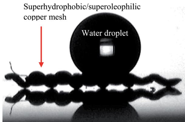
Fig. 8 Water droplet on a copper 60 mesh substrate with a coating D surface ( $\text{SiO}_2$  5–15  $\mu\text{m}$  particles (0.6 g) with  $\text{TiO}_2$  21 nm particles (0.6 g) in a 1 : 9 polymer mixture of Sylgard® 184 and FAS). Image was recorded post separation functional testing.
