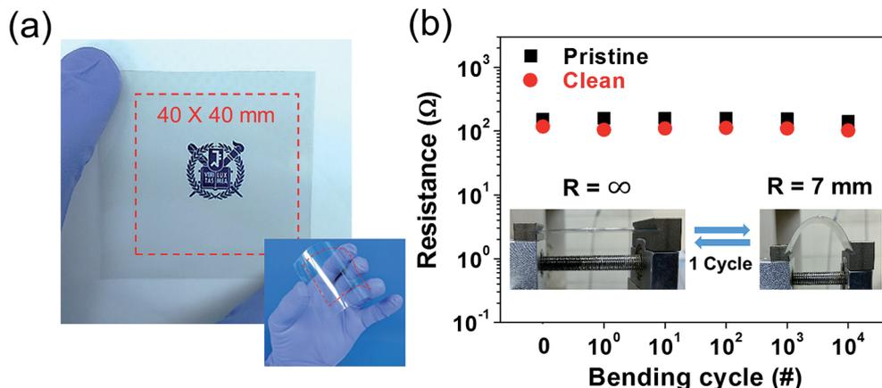
Fig. 7 (a) Photographic image of a graphene film transferred onto a flexible polyimide substrate ( $40 \times 40 \text{ mm}^2$ ). (b) The resistance of the graphene films on the flexible polyimide substrate under repeated bending cycles (0, 10, 100, 1000, and 10 000 times; bending radius = 5 mm).
