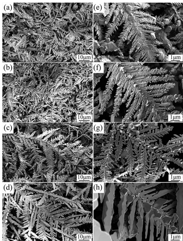
Fig. 1 SEM images of polished Cu substrate at different reaction times in an aqueous solution of  $\text{AgNO}_3$  under different magnifications: (a) and (e) 5 min, (b) and (f) 10 min, (c) and (g) 15 min, (d) and (h) 20 min.
