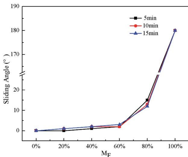
Fig. 5 Effects of reaction time and  $M_F$  on WSA for STA@Ag@Cu ( $M_F = 0\%$ ), PFOA@Ag@Cu ( $M_F = 100\%$ ) and 4 intermediate mixtures surfaces ( $M_F = 20\%$ , 40%, 60%, 80%).
