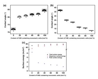
Fig. 6 (a) Water, (b) diiodomethane contact angle, and (c) surface energy values of PVAN# films according to the molar content of the vanilly butyl ether moiety in the side groups.
