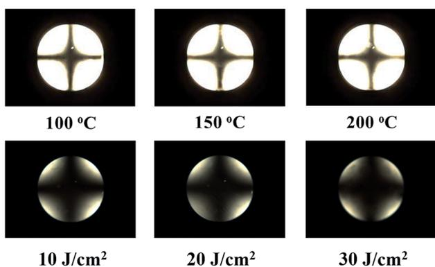
Fig. 7 Conoscopic POM images of the LC cells made from PVAN100 films, observed after external conditions; heat treatment at 100, 150, and 200 °C for 10 min and ultraviolet at 10, 20, and 30 J cm<sup>-2</sup>, respectively.
