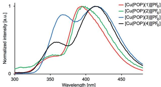
Fig. 11 Emission spectra for  $\text{CH}_2\text{Cl}_2$  solutions of  $[\text{Cu}(\text{POP})(\text{N}^{\wedge}\text{S})][\text{PF}_6]$  ( $5.0 \times 10^{-5}$  M).  $\lambda_{\text{exc}} = 275$  nm for 1, 250 nm for 2, 280 nm for 3, 270 nm for 4.
