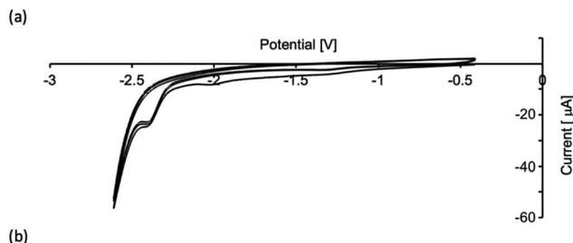
Fig. 5 Three successive scans in the cyclic voltammogram of  $[\text{Cu}(\text{xantphos})(4)][\text{PF}_6]$  in  $\text{CH}_2\text{Cl}_2$  (ca.  $2 \times 10^{-3}$  M, vs.  $\text{Fc}^+/\text{Fc}$ ,  $[\text{t}^{\text{Bu}}_4\text{N}][\text{PF}_6]$  as supporting electrolyte, scan rate =  $0.1 \text{ V s}^{-1}$ ): (a) oxidative scans to +1.2 V, (b) reductive scans to  $-2.6$  V.
