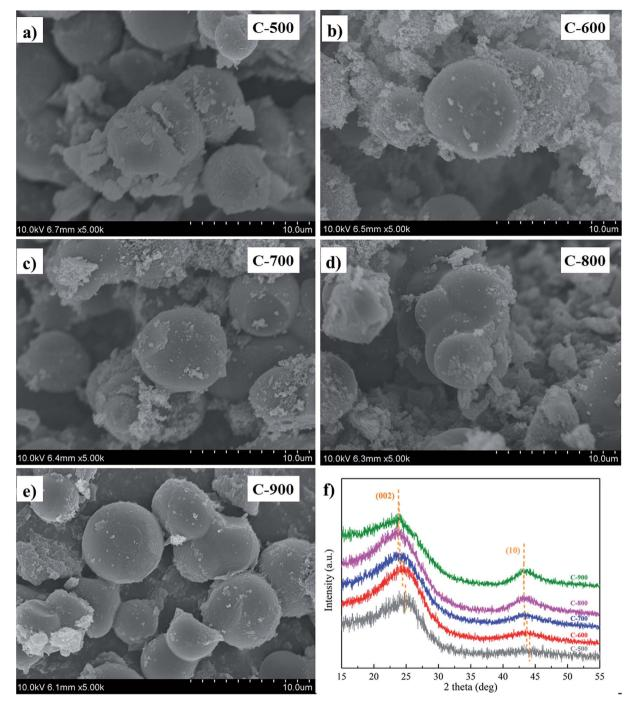
Fig. 1 SEM images (a-e) and XRD patterns (f) of the activated carbons
