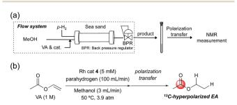
Fig. 7 (a) Illustration of flow hydrogenation system used in this study. (b) Reaction conditions for PHIP of VA in (a).
