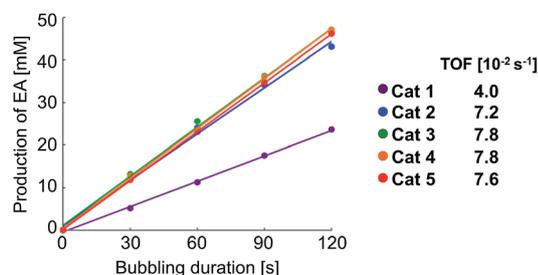
Fig. 4 TOF of Rh catalysts 1–5 in hydrogenation for vinyl acetate (VA). Determination of TOF for VA (cat 1–5). 5 mM of catalyst solution in methanol- $d_4$  containing 1 M of VA was set into an NMR tube, and bubbled with normal hydrogen (20 mL  $\text{min}^{-1}$ ).
