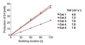
Fig. 4 TOF of Rh catalysts 1-5 in hydrogenation for vinyl acetate (VA). Determination of TOF for VA (cat 1-5). 5 mM of catalyst solution in methanol- $d_4$  containing 1 M of VA was set into an NMR tube, and bubbled with normal hydrogen (20 mL min<sup>-1</sup>).
