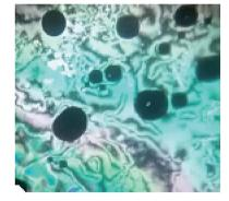
Fig. 4 Nematic mesophase texture under a polarized optical microscope for supramolecular complex IB at 126 °C upon heating.
