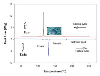
Fig. 2 DSC thermogram for I upon second heating/cooling cycles with heating rate 10 °C min<sup>-1</sup>
