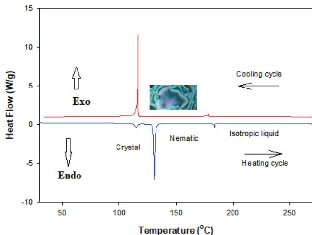
Fig. 2 DSC thermogram for **I** upon second heating/cooling cycles with heating rate  $10\text{ }^{\circ}\text{C min}^{-1}$ .
