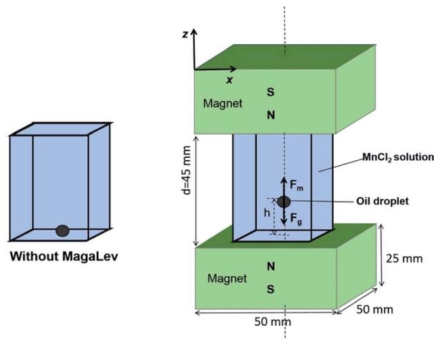
Fig. 1 Schematic representation of the experimental setup of magnetic levitation (MagLev). A container filled with  $\text{MnCl}_2$  solution was placed between two indistinguishable NdFeB magnets (50 mm  $\times$  50 mm  $\times$  25 mm), aligned vertically, 45 mm apart, with like poles facing each other. The droplet of cooking oil was levitated in the MagLev device due to the balance of the gravitational force,  $\vec{F}_{\text{g}}$ , and the magnetic force,  $\vec{F}_{\text{mag}}$ .
