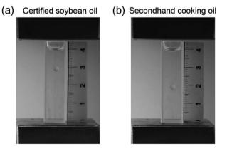
Fig. 6 Detection of secondhand cooking oil using MagLev. Photographs of the droplets of (a) certified soybean oil and (b) secondhand cooking oil levitated in the MagLev device.
