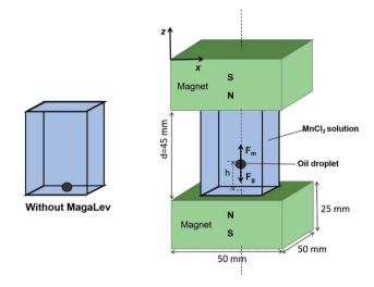
Fig. 1 Schematic representation of the experimental setup of magnetic levitation (MagLev). A container filled with MnCl<sub>2</sub> solution was placed between two indistinguishable NdFeB magnets (50 mm imes50 mm × 25 mm), aligned vertically, 45 mm apart, with like poles facing each other. The droplet of cooking oil was levitated in the MagLev device due to the balance of the gravitational force,  $\vec{F}_{
