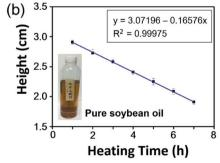
Fig. 4 Detection of heated pure soybean oil using MagLev. (a) Photographs of the droplets of pure soybean oil that was heated for 1 h, 2 h, 3 h, 4 h, 5 h, 6 h, and 7 h levitated in the MagLev device. (b) Plot correlating the levitation height of the droplets of pure soybean oil with the heating time. Each data point is the mean of five analyses.
