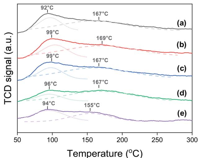
Fig. 2 CO<sub>2</sub>-TPD patterns of (a) Na<sub>0.2</sub>/Fe<sub>1</sub>Zn<sub>1.2</sub>O<sub>x</sub> (350), (b) Na<sub>0.2</sub>/Fe<sub>1</sub>Zn<sub>1.2</sub>O<sub>x</sub> (400), (c) Na<sub>0.2</sub>/Fe<sub>1</sub>Zn<sub>1.2</sub>O<sub>x</sub> (500), (d) Na<sub>0.2</sub>/Fe<sub>1</sub>Zn<sub>1.2</sub>O<sub>x</sub> (600), (e) Na<sub>0.2</sub>/Fe<sub>1</sub>Zn<sub>1.2</sub>O<sub>x</sub> (700).
