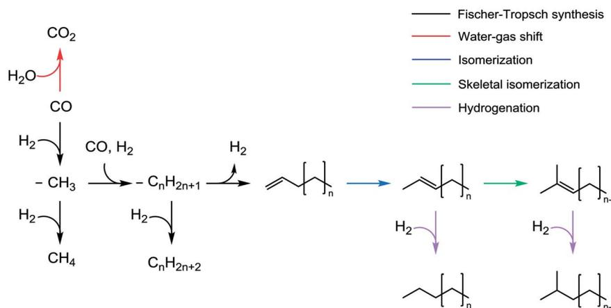
Fig. 8 Proposed secondary reaction pathways for Na-promoted catalysts.
