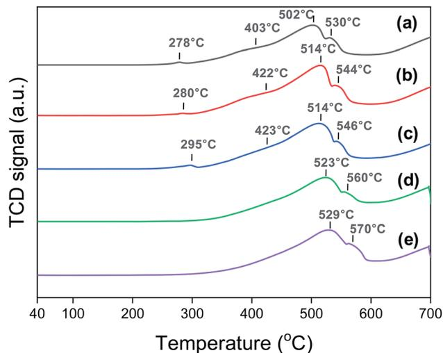
Fig. 3  $\text{H}_2$ -TPR patterns of (a)  $\text{Na}_{0.2}/\text{Fe}_1\text{Zn}_{1.2}\text{O}_x$  (350), (b)  $\text{Na}_{0.2}/\text{Fe}_1\text{Zn}_{1.2}\text{O}_x$  (400), (c)  $\text{Na}_{0.2}/\text{Fe}_1\text{Zn}_{1.2}\text{O}_x$  (500), (d)  $\text{Na}_{0.2}/\text{Fe}_1\text{Zn}_{1.2}\text{O}_x$  (600), (e)  $\text{Na}_{0.2}/\text{Fe}_1\text{Zn}_{1.2}\text{O}_x$  (700) before the reaction.
