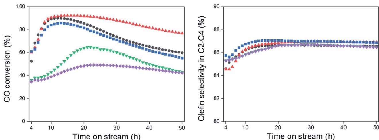
Fig. 4 CO conversion and olefin selectivity in C2–C4, (●)  $\text{Na}_{0.2}/\text{Fe}_1\text{Zn}_{1.2}\text{O}_x$  (350), (▲)  $\text{Na}_{0.2}/\text{Fe}_1\text{Zn}_{1.2}\text{O}_x$  (400), (■)  $\text{Na}_{0.2}/\text{Fe}_1\text{Zn}_{1.2}\text{O}_x$  (500), (▼)  $\text{Na}_{0.2}/\text{Fe}_1\text{Zn}_{1.2}\text{O}_x$  (600), (◆)  $\text{Na}_{0.2}/\text{Fe}_1\text{Zn}_{1.2}\text{O}_x$  (700).
