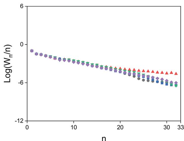
Fig. 6 Hydrocarbon molecular weight distribution for Na/Fe–Zn catalysts, (●)  $\text{Na}_{0.2}/\text{Fe}_1\text{Zn}_{1.2}\text{O}_x$  (350), (▲)  $\text{Na}_{0.2}/\text{Fe}_1\text{Zn}_{1.2}\text{O}_x$  (400), (■)  $\text{Na}_{0.2}/\text{Fe}_1\text{Zn}_{1.2}\text{O}_x$  (500), (▼)  $\text{Na}_{0.2}/\text{Fe}_1\text{Zn}_{1.2}\text{O}_x$  (600), (◆)  $\text{Na}_{0.2}/\text{Fe}_1\text{Zn}_{1.2}\text{O}_x$  (700).
