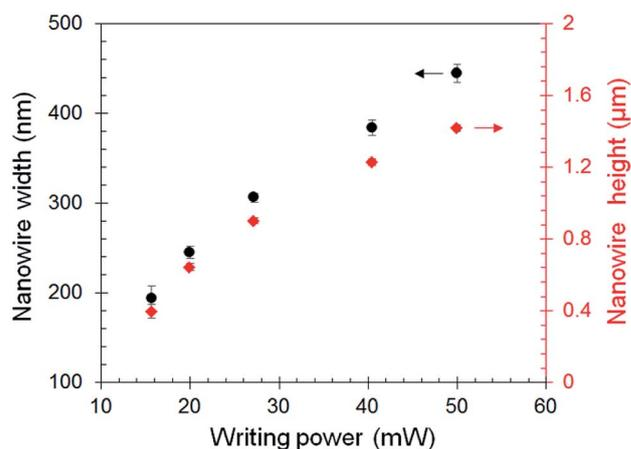
Fig. 3 Width and height of green-state nanowires versus the time-averaged laser power. Nanowires were written in IP-DIP resist at a writing speed of  $10 \text{ mm s}^{-1}$ . Time-averaged writing power of  $50 \text{ mW}$  for the beam corresponds to a peak intensity of  $2.43 \text{ TW cm}^{-2}$  at the center of the focused light spot. Error bars on width and height quantify the 1-standard deviation of the uncertainty across multiple nanowires printed under identical conditions.
