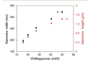
Fig. 3 Width and height of green-state nanowires *versus* the time-averaged laser power. Nanowires were written in IP-DIP resist at a writing speed of  $10~{\rm mm\,s^{-1}}$ . Time-averaged writing power of  $50~{\rm mW}$  for the beam corresponds to a peak intensity of  $2.43~{\rm TW~cm^{-2}}$  at the center of the focused light spot. Error bars on width and height quantify the 1-standard deviation of the uncertainty across multiple nanowires printed under identical conditions.
