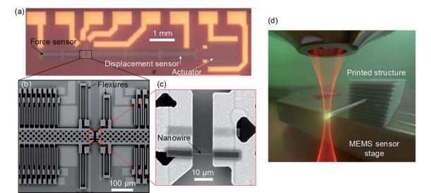
Fig. 1 Micro-electro-mechanical systems (MEMS)-based miniaturized tensile tester. (a) Optical image of the unpackaged tensile tester illustrating the actuator and the two sensors. (b and c) Scanning electron microscope images of the sensor pads and the polymer nanowire printed across the two stages. (d) Schematic representation of printing of a nanowire directly on top of a MEMS sensor via two-photon lithography.
