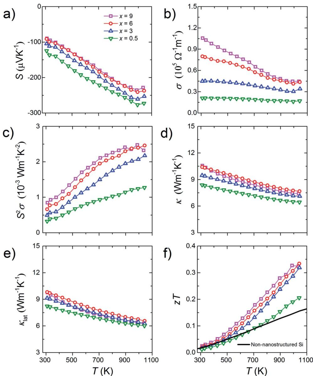
Fig. 5 Temperature dependences of (a) Seebeck coefficient,  $S$ , (b) electrical conductivity,  $\sigma$ , (c) power factor,  $S^2\sigma$ , (d) thermal conductivity,  $\kappa$ , (e) lattice thermal conductivity,  $\kappa_{\text{lat}}$  and (f) dimensionless figure of merit,  $zT$  of the bulk samples with the doping level of  $x\%$  molar parts to Si. The  $zT$  data for typical non-nanostructured n-type bulk  $\text{Si}^{17}$  are shown as a solid line for comparison.
