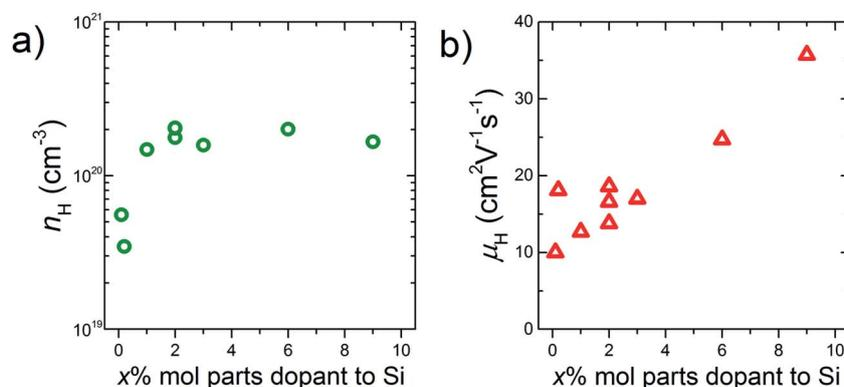
Fig. 4 (a) Carrier concentration,  $n_H$  and (b) mobility,  $\mu_H$ , as a function of the doping level, x% molar parts to Si. All the data are obtained at room temperature.
