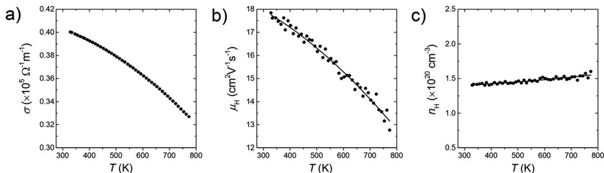
Fig. 6 Results of the high-temperature Hall measurement for a bulk sample whose doping level is 3% molar parts to Si. Temperature dependences of (a) electrical conductivity,  $\sigma$ , (b) Hall mobility,  $\mu_{\text{H}}$ , and (c) Hall carrier concentration,  $n_{\text{H}}$ . The solid lines are obtained by fitting the data points.
