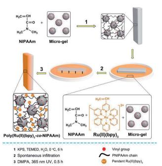
Fig. 1 Preparation method of the interpenetrating PNIPAAm/poly(Ru( $_{\rm II}$ )(bpy) $_{\rm 3}$ - $_{\rm co}$ -NIPAAm) double network gel (MG) with asymmetric distribution of Ru( $_{\rm II}$ )(bpy) $_{\rm 3}$ .
