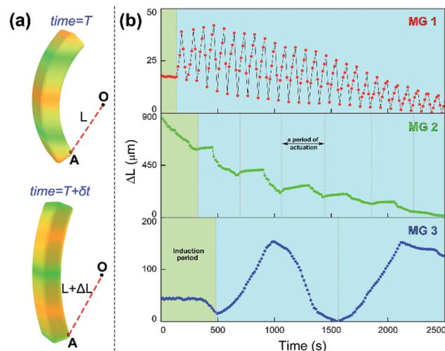
Fig. 3 Continuous cyclic actuation profiles of MGs in the solution of BZ substrates ([HNO<sub>3</sub>] = 0.89 M, [NaBrO<sub>3</sub>] = 84 mM, [MA] = 62.5 mM) at 20 °C. (a) Illustration of quantitative method. (b) Actuation profiles of MGs, the time interval of data collection is 15 s.
