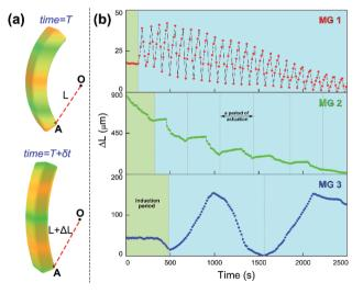
Fig. 3 Continuous cyclic actuation profiles of MGs in the solution of BZ substrates ( $[HNO_3] = 0.89 \text{ M}$ ,  $[NaBrO_3] = 84 \text{ mM}$ , [MA] = 62.5 mM) at 20 °C. (a) Illustration of quantitative method. (b) Actuation profiles of MGs, the time interval of data collection is 15 s
