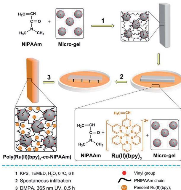
Fig. 1 Preparation method of the interpenetrating PNIPAAm/poly(Ru(II)(bpy)<sub>3</sub>-*co*-NIPAAm) double network gel (MG) with asymmetric distribution of Ru(II)(bpy)<sub>3</sub>.
