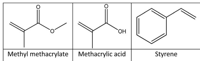
Fig. 8 Chemical structure of methyl methacrylate, methacrylic acid and styrene.
