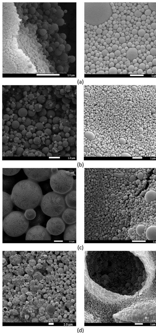
Fig. 6 Scanning electron microscopy (SEM) the copolymers capsules with (a) methacrylic acid/methyl methacrylate (MAA/MMA\_R.O.), (b) methacrylic acid/methyl methacrylate (MAA/MMA), (c) methacrylic acid/methyl methacrylate/styrene (MAA/MMA/STY\_R.O.) and (d) methacrylic acid/methyl methacrylate/styrene (MAA/MMA/STY).
