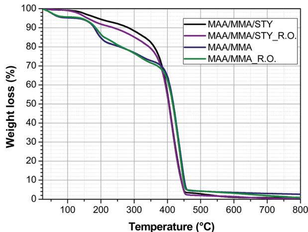
Fig. 10 Thermogravimetric analysis of methacrylic acid/methyl methacrylate copolymers (MAA/MMA), the capsules with methacrylic acid/methyl methacrylate (MAA/MMA\_R.O.) and methacrylic acid/methyl methacrylate/styrene (MAA/MMA/STY) and the methacrylic acid/methyl methacrylate/styrene terpolymers (MAA/MMA/STY\_R.O.).
