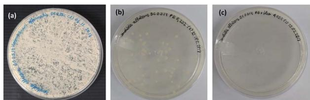
Fig. 12 *Candida albicans* fungus culture plates treated with (a) 0.25% essential oil of *Rosmarinus officinalis*, (b) 0.25% of methacrylic acid/methyl methacrylate/styrene terpolymer (MAA/MMA/STY) (c) 0.25% of methacrylic acid/methyl methacrylate/styrene terpolymer with the encapsulated essential oil (MAA/MMA/STY\_R.O.).
