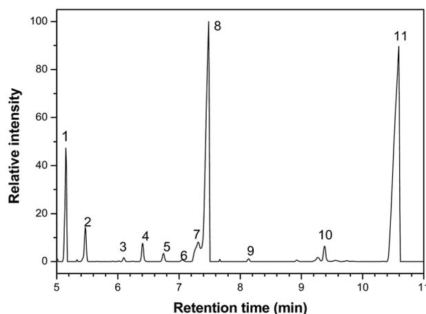
**Fig. 1** Chromatogram obtained by gas chromatography-mass spectrometry analysis of *Rosmarinus officinalis* essential oil, where the numbers from 1 to 11 correspond to the majority components, whose names are shown in the Table 4.
