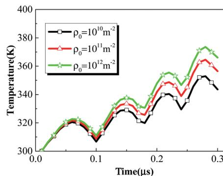
Fig. 19 Volume averaged temperature histories of rodlike samples with initial dislocation density of  $1 \times 10^{10} \text{ m}^{-2}$ ,  $1 \times 10^{11} \text{ m}^{-2}$ , and  $1 \times 10^{12} \text{ m}^{-2}$ .
