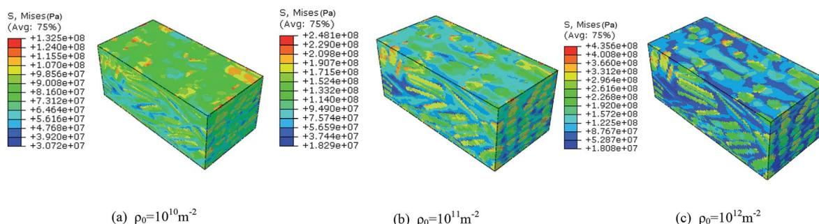
Fig. 15 Von Mises stress contours of rodlike samples with initial dislocation density of: (a)  $1 \times 10^{10} \text{ m}^{-2}$ , (b)  $1 \times 10^{11} \text{ m}^{-2}$ , and (c)  $1 \times 10^{12} \text{ m}^{-2}$ .
