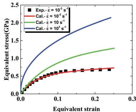
Fig. 1 Calibration of constitutive model of LLM-105.
