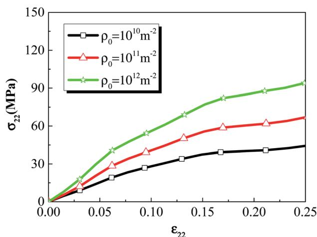
Fig. 14 Volume averaged stress strain curves of rodlike samples with initial dislocation density of  $1 \times 10^{10} \text{ m}^{-2}$ ,  $1 \times 10^{11} \text{ m}^{-2}$ , and  $1 \times 10^{12} \text{ m}^{-2}$ .
