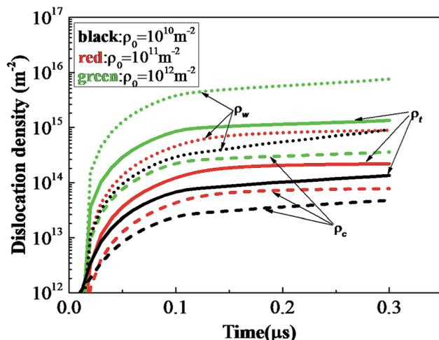
Fig. 17 Total dislocation density  $\rho_t$  (solid curves), dislocation density at crystal wall  $\rho_w$  (dotted curves) and dislocation density at crystal interior  $\rho_c$  (dashed curves) histories of rodlike samples with initial dislocation density of  $1 \times 10^{10} \text{ m}^{-2}$ ,  $1 \times 10^{11} \text{ m}^{-2}$ , and  $1 \times 10^{12} \text{ m}^{-2}$ .
