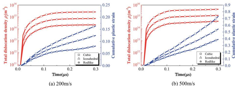
Fig. 6 Volume averaged total dislocation density (red curves) and cumulative plastic strain histories (blue curves) of cubic, icosahedral and rodlike samples at an impact velocity of (a)  $200 \text{ m s}^{-1}$  and (b)  $500 \text{ m s}^{-1}$ .
