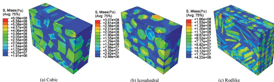
Fig. 4 Von Mises stress contour at  $t = 3 \mu\text{s}$  of cubic, icosahedral and rodlike samples at an impact velocity of 200 m s<sup>-1</sup>.
