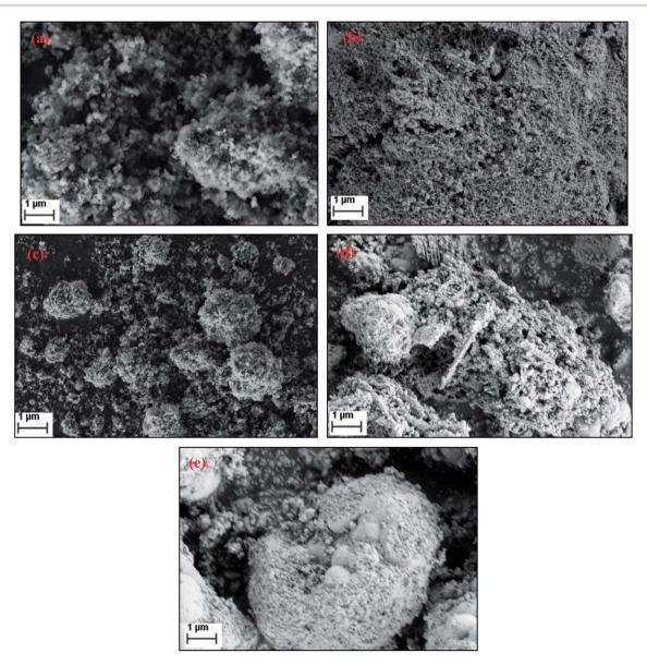
Fig. 5 Scanning electron micrographs (SEM) of FePO<sub>4</sub> catalysts under various conditions (a) fresh, (b) reduced under CH<sub>4</sub>, (c) oxidized with O<sub>2</sub>, (d) oxidized with N2O and (e) oxidized with H2O.
