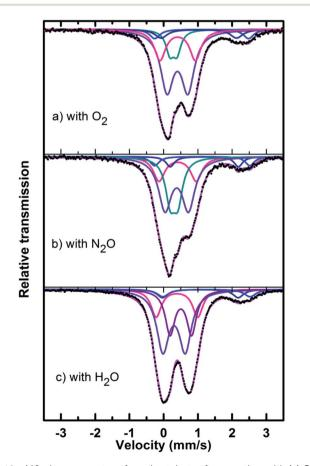
Fig. 10 Mössbauer spectra of used catalysts after reaction with (a)  $O_2$ , (b)  $N_2O$  and (c)  $H_2O$ .
