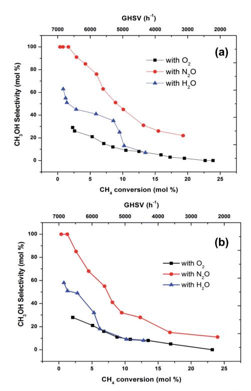
Fig. 3 Selectivity towards methanol varying with methane conversion over FePO<sub>4</sub> catalyst at the temperatures of (a) 300 °C and (b) 400 °C (GHSV =  $2000-7000 \text{ h}^{-1}$ , methane to oxidant ratio of 1 : 1).
