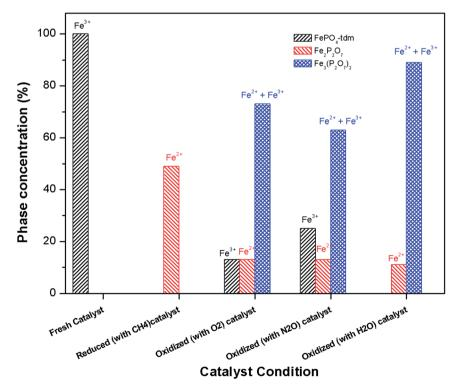
Fig. 9 Phase quantification of fresh, reduced (with CH<sub>4</sub>) and oxidized (with N<sub>2</sub>O, O<sub>2</sub> and H<sub>2</sub>O) FePO<sub>4</sub> catalyst determined from the Mössbauer spectra shown in Fig. 8.
