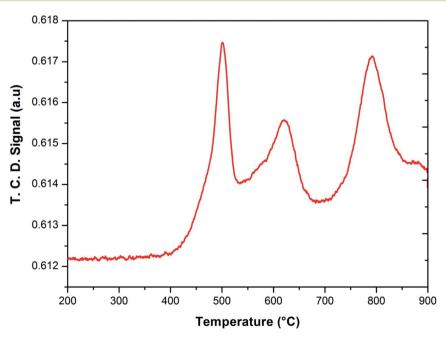
Fig. 6 Temperature programmed reduction of FePO<sub>4</sub> catalyst under 10% CH<sub>4</sub> in Ar.
