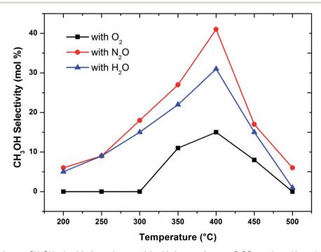
Fig. 2 Influence of oxidant on CH<sub>3</sub>OH selectivity in methane partial oxidation reaction over FePO<sub>4</sub> catalyst with varying temperature (GHSV =  $3600 \text{ h}^{-1}$  and methane to oxidant ratio of 1 : 1).
