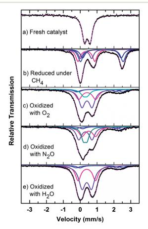
Fig. 8 Mössbauer spectra of fresh, reduced (with  $CH_4$ ) and oxidized (with  $N_2O$ ,  $O_2$  and  $H_2O$ ) FePO $_4$  catalyst.
