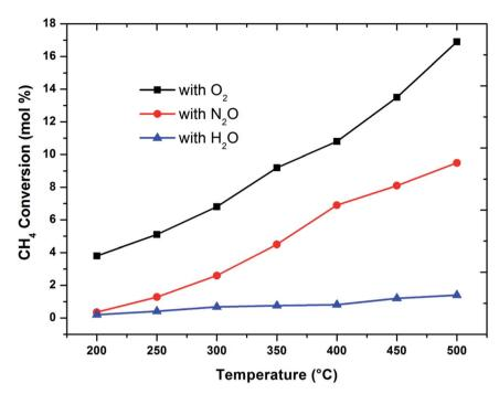
Fig. 1 Influence of oxidant on methane conversion over FePO<sub>4</sub> catalyst with varying temperature (GHSV =  $3600 \text{ h}^{-1}$  and methane to oxidant ratio of 1 : 1).
