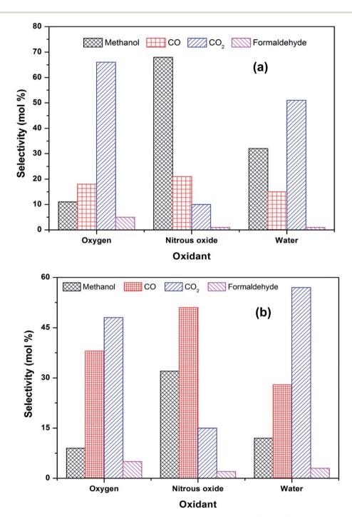
Fig. 4 Selectivity towards products in the partial oxidation of methane at an iso-conversion of (a) 5% and (b) 10% over FePO<sub>4</sub> catalyst with various oxidants (temperatures of 400 °C and methane to oxidant ratio of 1:1).
