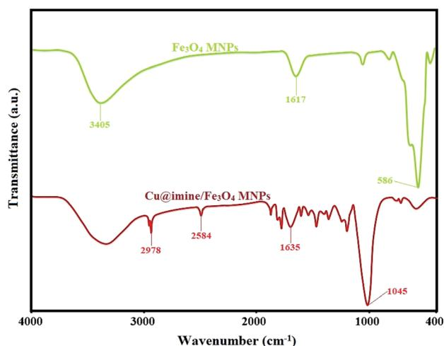
Fig. 1 FT-IR spectra of Fe<sub>3</sub>O<sub>4</sub> and Cu@imine/Fe<sub>3</sub>O<sub>4</sub> MNPs.
