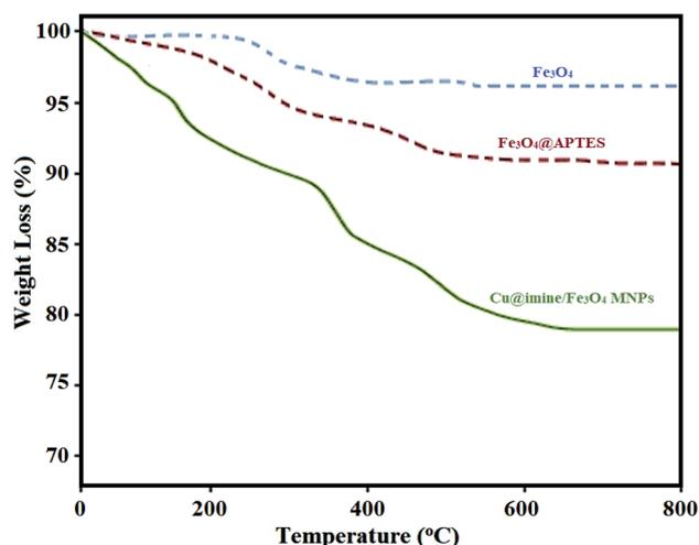
Fig. 2 TGA thermogram of Fe<sub>3</sub>O<sub>4</sub>, Fe<sub>3</sub>O<sub>4</sub>@APTES, Cu@imine/Fe<sub>3</sub>O<sub>4</sub> MNPs.
