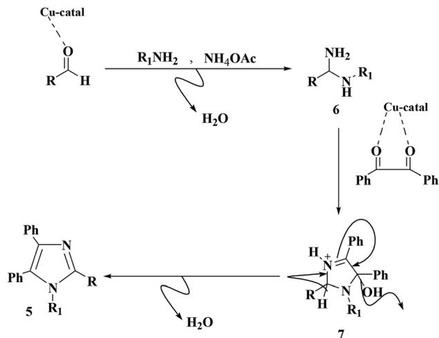
Scheme 2 A plausible mechanism of the creation of 1,2,4,5-tetra-substituted imidazoles derivatives in the existence of Cu@imine/Fe<sub>3</sub>O<sub>4</sub> MNPs under solvent-free conditions.
