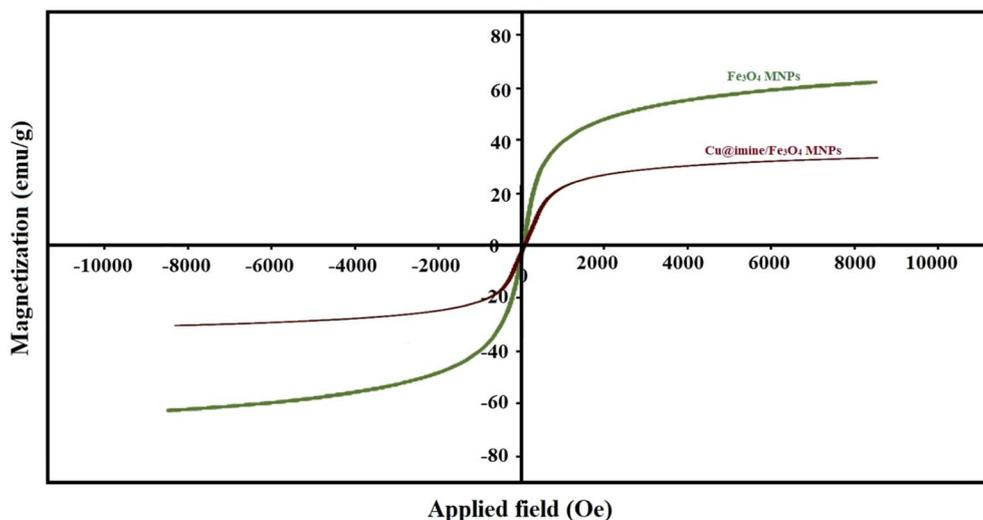
Fig. 3 Magnetization curves of  $\text{Fe}_3\text{O}_4$  and  $\text{Cu@imine/Fe}_3\text{O}_4$  MNPs.
