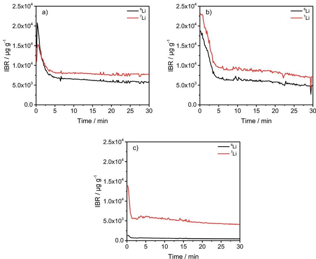
Fig. 3 IBRs for the  $^6\text{Li}$  and  $^7\text{Li}$  signals of differently aged, discharged anodes. (a) one formation step with C/5; (b) three formation steps with C/5 plus ten additional cycles with C/1; (c) one formation step with C/5 and the reference electrolyte cycled using the same procedure as the enriched cells for one formation step.
