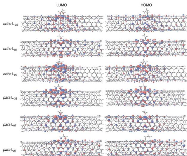
Fig. 4 Frontier molecular orbital diagrams of *ortho* and *para* adducts for SWNT-(C<sub>3</sub>H<sub>6</sub>) (B3LYP/6-31G\*, isovalue = 0.02).
