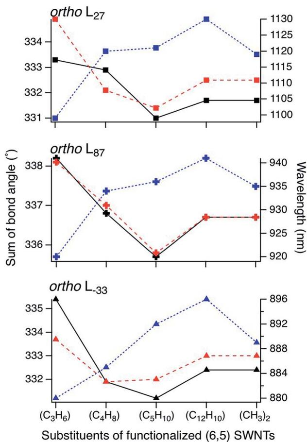
Fig. 3 Sum of bond angles at the addition sites in functionalized (6,5) SWNTs (black lines represent the addition position "a", and red lines represent the other addition position in *ortho* adducts). Calculated absorption energy of functionalized (6,5) SWNTs (blue line) using TD-DFT with B3LYP/3-21G. Different orientations in *ortho* adducts are marked in the same manner as in Fig. 2.
