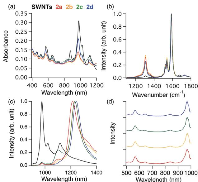
**Fig. 1** (a) Absorption spectra of **2** dispersed in a D<sub>2</sub>O solution containing 1 wt% SDBS. (b) Raman spectra of **2** (film) excited at 561 nm. Black: SWNTs. (c) Normalized PL spectra excited at 567 nm of **2** dispersed in a D<sub>2</sub>O solution containing 1 wt% SDBS. (d) Normalized excitation spectra of **2**. Red: **2a**, 1215 nm. Yellow: **2b**, 1230 nm. Green: **2c**, 1231 nm. Blue: **2d**, 1242 nm.
