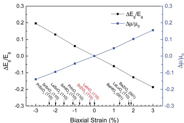
Fig. 6 The variations of band gap and electron mobility of strained  $\text{BaSnO}_3$  in comparison to the strain-free  $\text{BaSnO}_3$  as a function of biaxial strain. Some commercially available substrate materials are marked on the figure.
