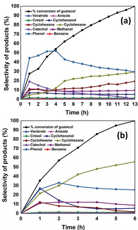
Fig. 2 Conversion (mol%) of guaiacol and selectivities of liquid products produced (mol%) with respect to increase in reaction time with (a) NiMoS<sub>2</sub>/AC and (b) NiMoS<sub>2</sub>/CMK-3 catalysts.
