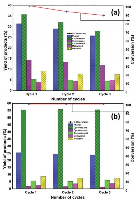
Fig. 4 The selectivities of liquid products (mol%) and the conversion of guaiacol by NiMoS<sub>2</sub>/AC and NiMoS<sub>2</sub>/CMK-3 catalysts for three cycles.
