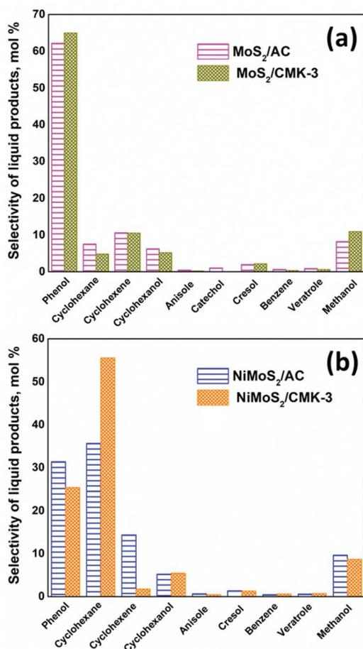
Fig. 1 Comparison of the selectivities of liquid products (mol%) by (a) MoS<sub>2</sub>/AC and MoS<sub>2</sub>/CMK-3 catalysts (b) NiMoS<sub>2</sub>/AC and NiMoS<sub>2</sub>/CMK-3 catalysts for the conversion of guaiacol after complete conversion.
