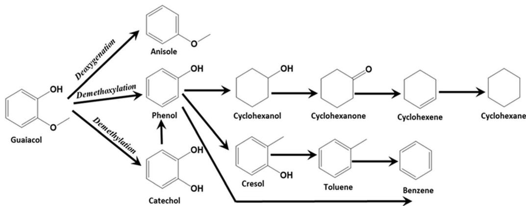
Scheme 1 Reaction network of hydrodeoxygenation of guaiacol by carbon supported NiMoS<sub>2</sub> catalyst.
