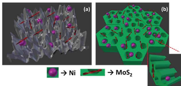
Fig. 3 Figure illustrating the Ni and MoS<sub>2</sub> active phase distribution over (a) activated carbon (b) CMK-3 supports.
