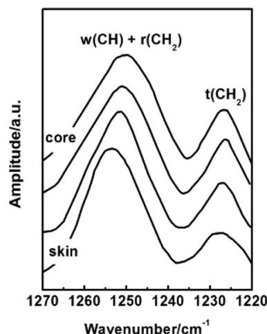
Fig. 11 Nano IR spectra of PAN fibres acquired in different radial position.
