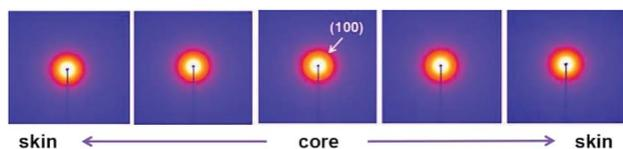
Fig. 4 2D-WAXD patterns of PAN fibres acquired in different radial positions.
