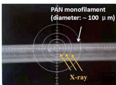
Fig. 1 Schematic of the measurement of micro-beam WAXD.
