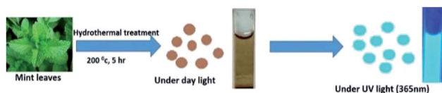
Fig. 1 Schematic representation of cyan luminescent CDs achieved from mint leaves.
