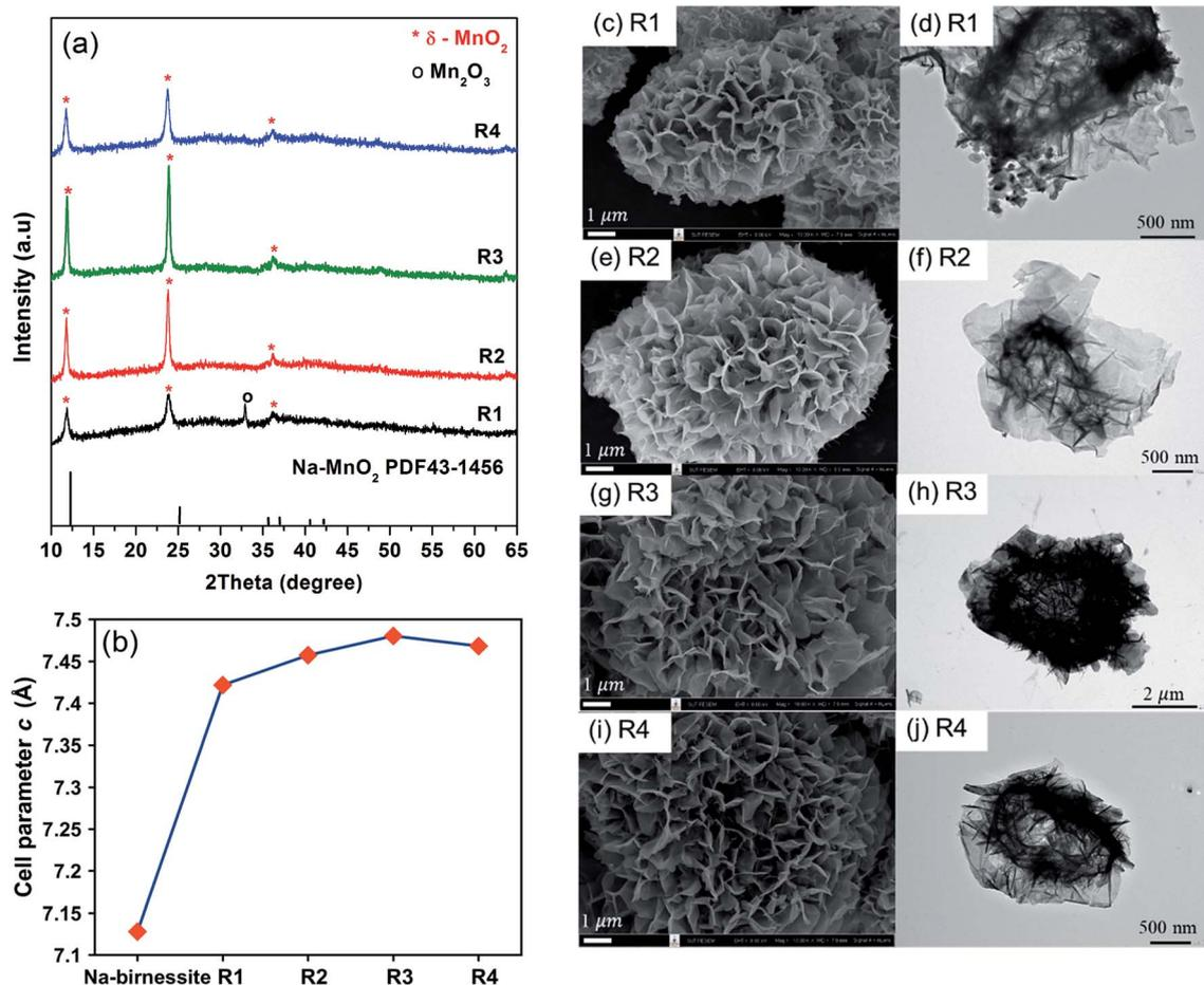
Fig. 3 XRD patterns (a) cell parameters, (b) SEM and TEM images, and (c–j) of Cs–MnO<sub>2</sub> obtained from molten salt synthesis with CsNO<sub>3</sub> : MnSO<sub>4</sub> weight ratios of 3 : 1 (R1), 5 : 1 (R2), 7 : 1 (R3), and 10 : 1 (R4) at 430 °C for 3 hours.
