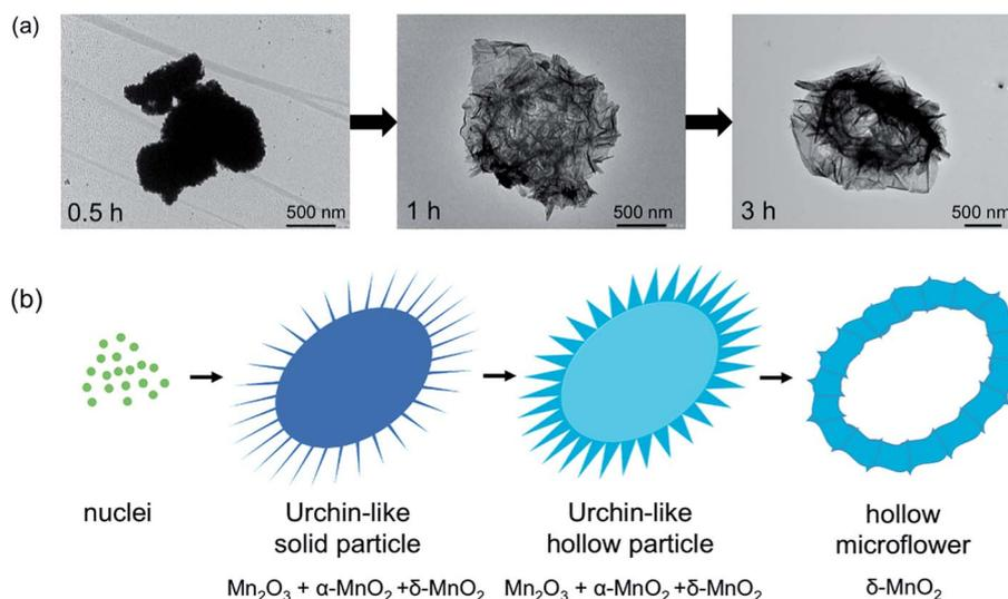
Fig. 2 TEM images (a), and formation process (b) of the products from molten salt synthesis.  $\delta\text{-MnO}_2$  formation occurs through formation of  $\text{Mn}_2\text{O}_3$  and  $\alpha\text{-MnO}_2$ , respectively. Simultaneously, the morphology changes from solid urchin-like particles to hollow microflowers as explained by Ostwald ripening process.
