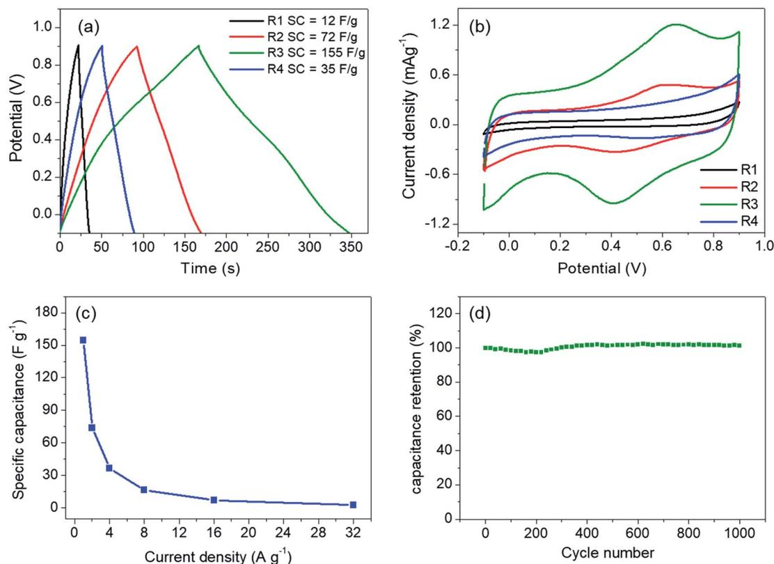
Fig. 5 (a) GCD curves at 1 A g<sup>-1</sup> and cyclic voltammograms at 5 mV s<sup>-1</sup> (b) of the samples obtained from molten salt synthesis with CsNO<sub>3</sub> : MnSO<sub>4</sub> weight ratios of 3 : 1 (R1), 5 : 1 (R2), 7 : 1 (R3), and 10 : 1 (R4). (c) and (d) show rate capability and cyclic performance at 5 A g<sup>-1</sup> of R3, respectively.
