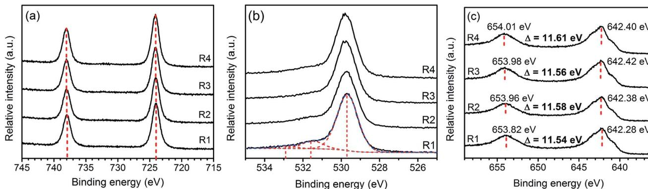
Fig. 4 XPS spectra: Cs3d (a), O2p (b), and Mn2p (c) of Cs-MnO<sub>2</sub> obtained from molten salt synthesis with CsNO<sub>3</sub> : MnSO<sub>4</sub> weight ratios of 3 : 1 (R1), 5 : 1 (R2), 7 : 1 (R3), and 10 : 1 (R4).
