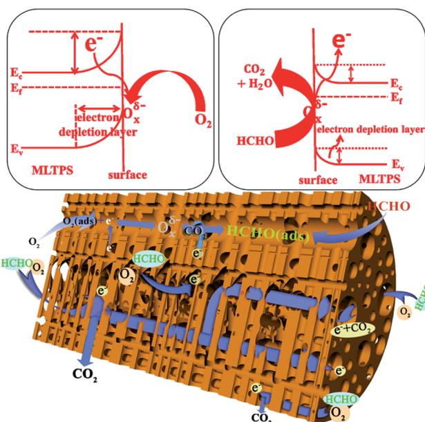
Fig. 9 Schematic of the gas sensing mechanism.
