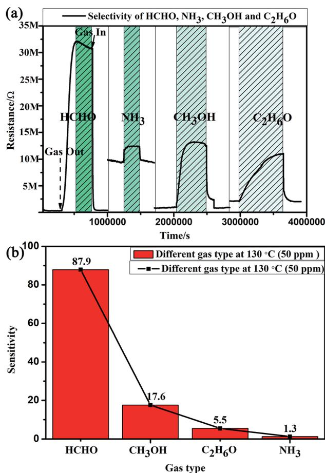
Fig. 7 Selectivity of the MLTPS gas sensor to 50 ppm HCHO, CH<sub>3</sub>OH, C<sub>2</sub>H<sub>6</sub>O and NH<sub>3</sub> at 130 °C. (a) The response and recovery curves of the different gases. (b) The responses of MLTPS to different gases.
