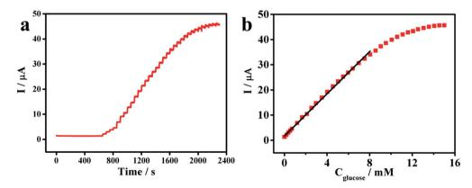
Fig. 4 (a) Amperometic responses of the PNE/GOD/AuNPs@PNE/Au electrode in PBS (pH 7.4) of 1 mM BQ at 0.7 V with successive additions of glucose; (b) calibration curve of the PNE/GOD/AuNPs@PNE/Au electrode with BQ.
