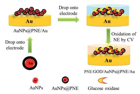
Scheme 1 Schematic illustration of the fabrication of the PNE/GOD/AuNPs@PNE/Au electrode.
