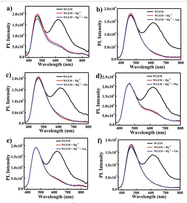
Fig. 7 Fluorescence intensity change of WLEM with Hg<sup>2+</sup> ions in presence of different amino acids (a) alanine; (b) aspartic acid; (c) histidine; (d) phenylalanine; (e) arginine; and (f) glutamic acid.
