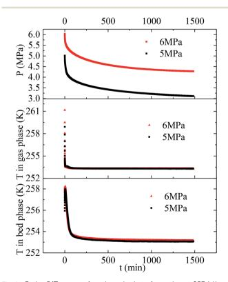
Fig. 1 Entire P/T curves of methane hydrate formation at 253.1 K and different original pressures of 5 and 6 MPa.
