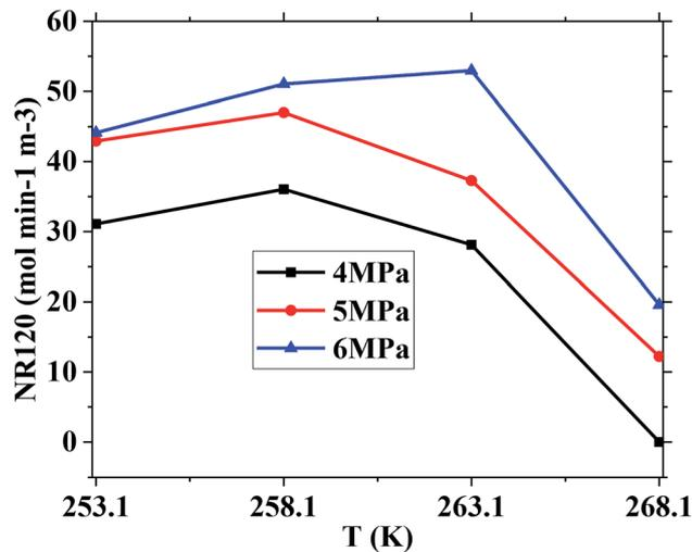
Fig. 4 The effect of temperature and pressure on  $NR_{120}$ .
