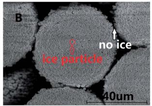
Fig. 6 The pictures observed by SEM for pore-saturated silica gel.
