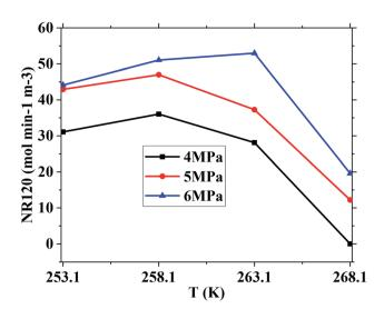
Fig. 4 The effect of temperature and pressure on NR<sub>120</sub>
