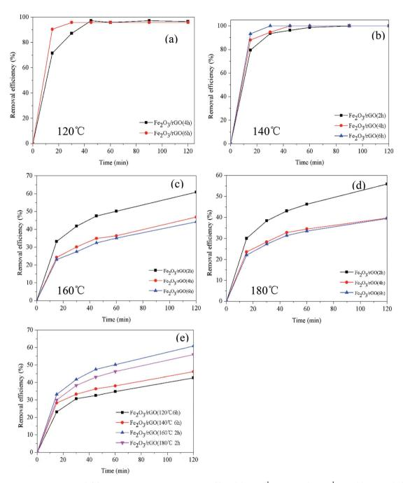
Fig. 1 Effect of preparation time on Cr(vi) removal at different temperatures ( $C_0 = 2.0 \text{ mg L}^{-1}$ ; dosage  $= 0.5 \text{ g L}^{-1}$ ; V = 100 mL; t = 2 h) (a) and (b); ( $C_0 = 5.0 \text{ mg L}^{-1}$ ; dosage  $= 0.2 \text{ g L}^{-1}$ ; V = 100 mL; t = 2 h) (c) and (d); comparison of the best samples in each group (e) ( $C_0 = 5.0 \text{ mg L}^{-1}$ ; dosage  $= 0.2 \text{ g L}^{-1}$ ; V = 100 mL; t = 2 h).
