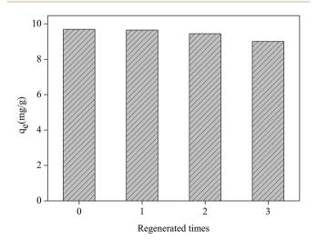
Fig. 10 Regeneration test of the  $Fe_2O_3/rGO$  (dosage = 0.2 g  $L^{-1}$ ;  $C_0$  = 5.0 mg L<sup>-1</sup>; V = 50 mL;  $t_{removal} = 3$  h; 0.1 mol L<sup>-1</sup> NaOH, desorption agent;  $t_{desorption} = 3 \text{ h}$ ).
