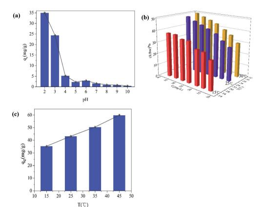
Fig. 9 Effect of pH on Cr(vi) removal ( $C_0 = 16.63 \text{ mg L}^{-1}$ ; dose of Fe<sub>2</sub>O<sub>3</sub>/rGO = 0.4 g L<sup>-1</sup>;  $T = 25 \pm 1 \,^{\circ}\text{C}$ ; t = 36 h; 140 rpm) (a); effect of the initial Cr(vi) concentration (b); effect of the temperatures (c) (dose of  $Fe_2O_3/rGO = 0.4 \text{ g L}^{-1}$ ; pH = 2.2; t = 36 h; 140 rpm).
