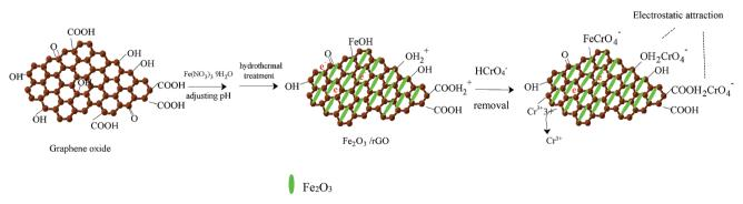
Schematic illustration for the preparation of Fe<sub>2</sub>O<sub>3</sub>/rGO and removal mechanism.
