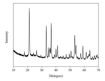
Fig. 4 The XRD pattern of Fe<sub>2</sub>O<sub>3</sub>/rGO.
