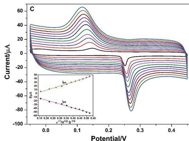
Fig. 4 (A) Cyclic voltammograms of  $4.0 \mu\text{M Cu}^{2+}$  in  $0.1 \text{ M PBS}$  (pH 6.5) at different scan rates on PG/GCE. (B) Cyclic voltammograms of  $4.0 \mu\text{M Cd}^{2+}$  in  $0.1 \text{ M PBS}$  (pH 6.5) at different scan rates on PG/GCE. (C) Cyclic voltammograms of  $2.0 \mu\text{M Hg}^{2+}$  in  $0.1 \text{ M PBS}$  (pH 6.5) at different scan rates on PG/GCE. Inset: plot of peak currents ( $I_{pa}$  and  $I_{pc}$ ) against the scan rate ( $\nu$ ).
