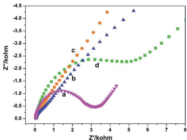
Fig. 2 EIS of (a) bare GCE, (b) PG/GCE, (c) GO/GCE, and (d) PGA/GCE in supporting electrolyte. Supporting electrolyte: 10 mmol  $\text{L}^{-1}$   $\text{K}_3[\text{Fe}(\text{CN})_6]/\text{K}_4[\text{Fe}(\text{CN})_6]$  (1 : 1) + 0.1 mol  $\text{L}^{-1}$  KCl solution.
