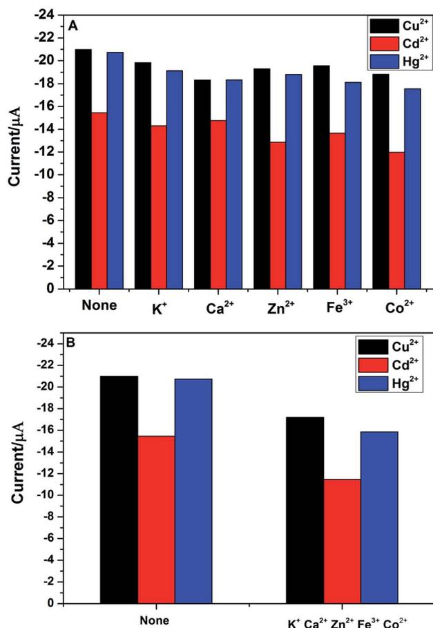
Fig. 7 (A) Effect of each interfering metal ions on detection of 2.0  $\mu\text{M}$   $\text{Cu}^{2+}$ ,  $\text{Cd}^{2+}$  and  $\text{Hg}^{2+}$  in 0.1 M PBS (pH 6.5). (B) Effect of five interfering metal ions on detection of 2.0  $\mu\text{M}$   $\text{Cu}^{2+}$ ,  $\text{Cd}^{2+}$  and  $\text{Hg}^{2+}$  in 0.1 M PBS (pH 6.5).
