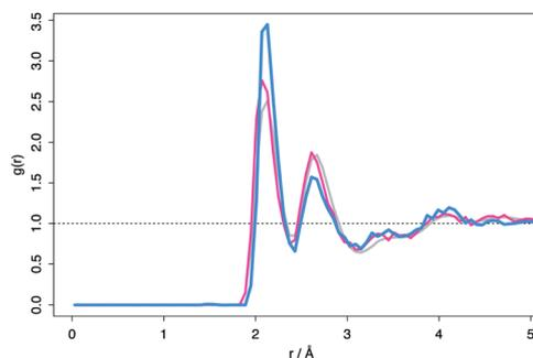
Fig. 3 Radial distribution functions,  $g(r)$ , of simulated amorphous zirconia (where  $r$  is atomic separation). Grey data: full amorphous structure obtained through molecular dynamics. Pink data: average data from  $20 \times 96$  atom cells produced through RMC technique. Blue data: average RDF for the 15 lowest energy relaxed supercells obtained through DFT.
