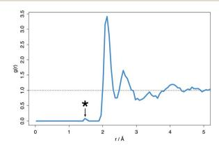
Fig. 8 Average radial distribution function (RDF) for the hyper-stoichiometric  $ZrO_2$  system after DFT structural minimization. \*Indicates the peak at 1.49 Å typical of the peroxide ion.
