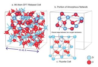
Fig. 4 An example of a DFT relaxed amorphous  $ZrO_2$  cell. A section of the amorphous network corresponding to the outlined atoms from (a) is shown in sub-figure (b). This shows that the network is primarily composed of oxygen tetrahedra in edge sharing configurations. The dashed lines indicate the position of these shared edges. Sub-figure (c) shows that this edge sharing topology is also evident in the crystal polymorphs of zirconia.
