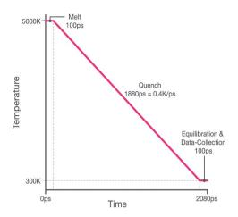
Fig. 1 Graphical representation melt-quench procedure.
