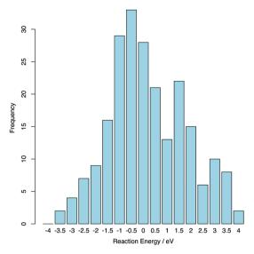
Fig. 7 Histogram illustrating the reaction energy for  $O_2$  to enter the amorphous  $ZrO_2$  supercells.
