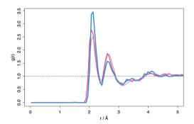
Fig. 3 Radial distribution functions, g(r), of simulated amorphous zirconia (where r is atomic separation). Grey data: full amorphous structure obtained through molecular dynamics. Pink data: average data from  $20 \times 96$  atom cells produced through RMC technique. Blue data: average RDF for the 15 lowest energy relaxed supercells obtained through DFT.
