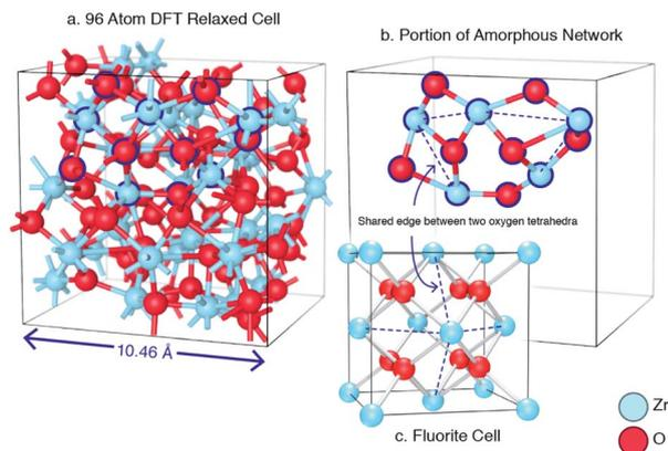
Fig. 4 An example of a DFT relaxed amorphous  $\text{ZrO}_2$  cell. A section of the amorphous network corresponding to the outlined atoms from (a) is shown in sub-figure (b). This shows that the network is primarily composed of oxygen tetrahedra in edge sharing configurations. The dashed lines indicate the position of these shared edges. Sub-figure (c) shows that this edge sharing topology is also evident in the crystal polymorphs of zirconia.
