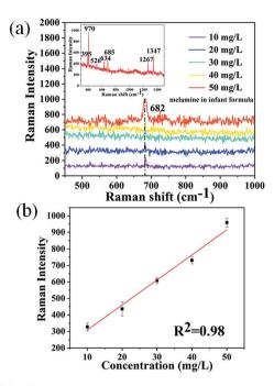
Fig. 4 (a) SERS spectra of melamine solution added into infant formula with a concentration ranging from 10 mg  $L^{-1}$  to 50 mg  $L^{-1}$ . The inset shows the Raman spectra of infant formula powder. (b) Average values with error bars calculated from the peak intensity at 682 cm<sup>-1</sup> versus different concentration of melamine in infant formula in (a).
