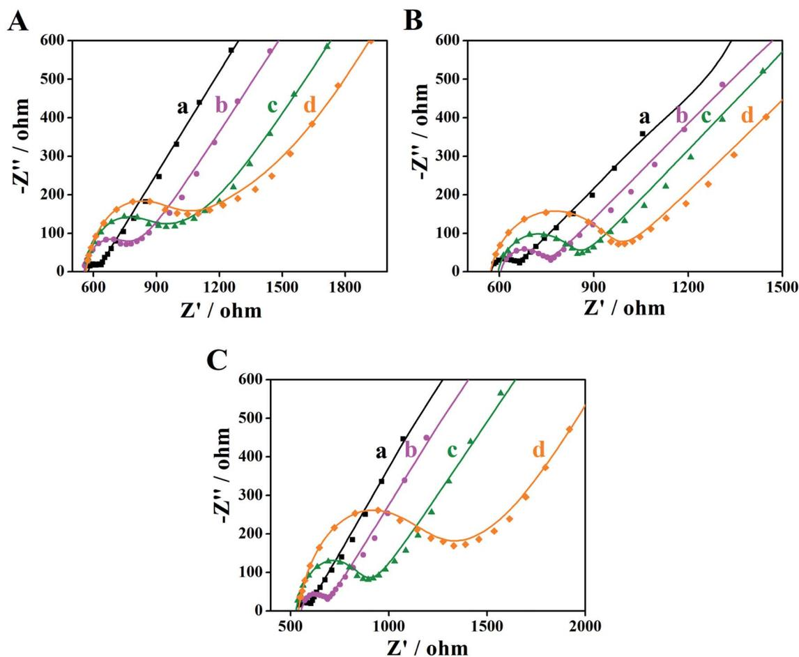
Fig. 8 EIS plots to trace the whole procedure of the CEA detection using the developed aptasensor based on (A) Au/NCNT/AE, (B) Au/PU-NCNT/AE, and (C) Au/FU-NCNT/AE, respectively, in 5 mM  $[\text{Fe}(\text{CN})_6]^{3-/4-}$  containing 0.14 M NaCl and 0.1 M KCl. (A): (a) AE, (b) Au/NCNT/AE, (c) Apt/Au/NCNT/AE, (d) CEA/Apt/Au/NCNT/AE; (B): (a) AE, (b) Au/PU-NCNT/AE, (c) Apt/Au/PU-NCNT/AE, (d) CEA/Apt/Au/PU-NCNT/AE; (C): (a) AE, (b) Au/FU-NCNT/AE, (c) Apt/Au/FU-NCNT/AE, (d) CEA/Apt/Au/FU-NCNT/AE.
