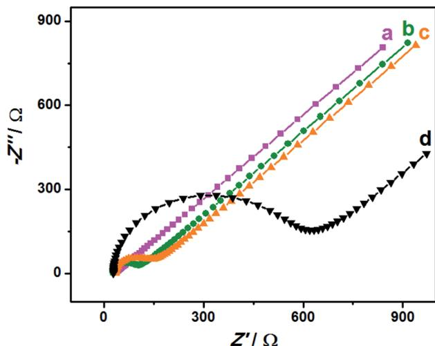
Fig. 4 EIS for 5.0 mM  $[\text{Fe}(\text{CN})_6]^{3-/4-}$  in 0.1 M KCl: (a) Au/NCNT/GCE, (b) Au/PU-NCNT/GCE, (c) Au/FU-NCNT/GCE and (d) bare GCE, frequency ranges: 0.1– $10^5$  Hz.
