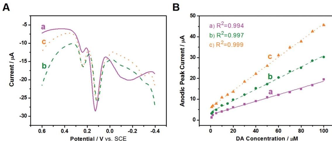
Fig. 7 (a) Au/NCNT/GCE, (b) Au/PU-NCNT/GCE, and (c) Au/FU-NCNT/GCE: (A) DPVs of 50  $\mu\text{M}$  DA, 50  $\mu\text{M}$  UA and 300  $\mu\text{M}$  AA in 0.1 M PBS (pH 7.4). (B) Linear relationship between the anodic peak current and the concentration of DA.
