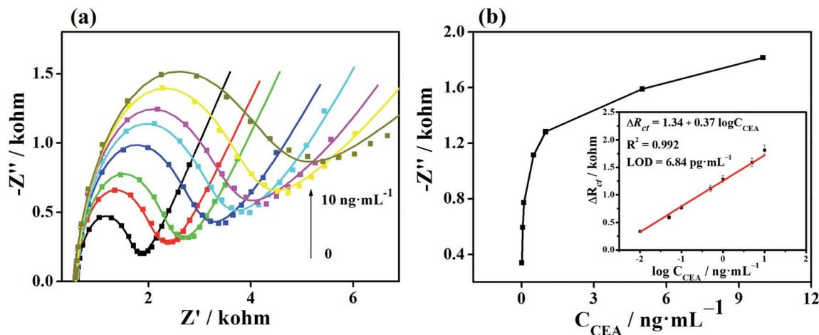
Fig. 9 (a) EIS responses of the Au/FU-NCNT/AE with different CEA concentrations (0, 0.01, 0.05, 0.1, 0.5, 1, 5, and 10 ng mL<sup>-1</sup>). (b) Dependence of  $\Delta R_{ct}$  on the concentration of CEA. The linear part of the calibration curve is shown in the inset of (b).
