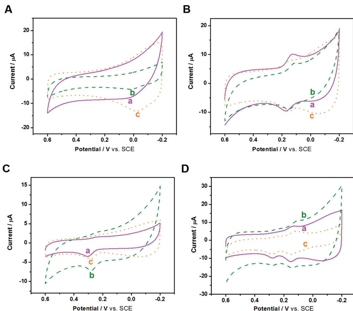
Fig. 6 CVs of (A) 300  $\mu\text{M}$  AA, (B) 50  $\mu\text{M}$  DA, (C) 50  $\mu\text{M}$  UA, and (D) mixture of 50  $\mu\text{M}$  DA, 50  $\mu\text{M}$  UA, 300  $\mu\text{M}$  AA at (a) Au/NCNT/GCE, (b) Au/PU-NCNT/GCE, and (c) Au/FU-NCNT/GCE in 0.1 M PBS (pH 7.4). Scan rate: 100  $\text{mV s}^{-1}$ .
